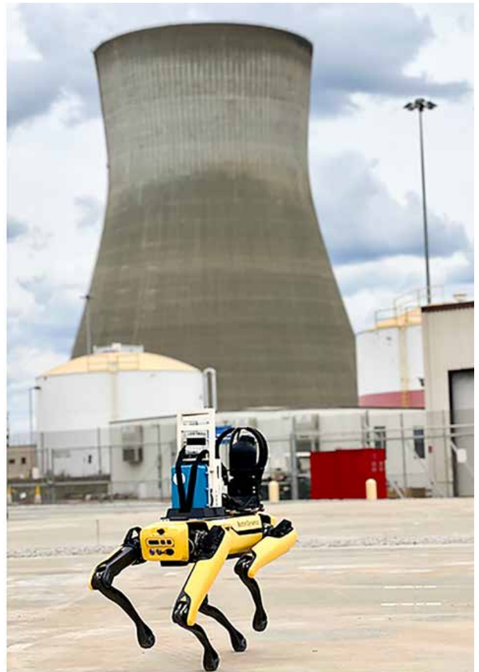
Figure 9: Example of imaging system installed on quadrupedal robotic platform during a routine assay.
