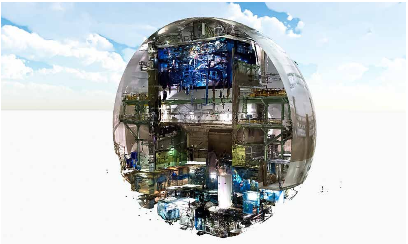
Figure 2: Point cloud of a Boiling Water Reactor building. Courtesy of Nucleco spa.
