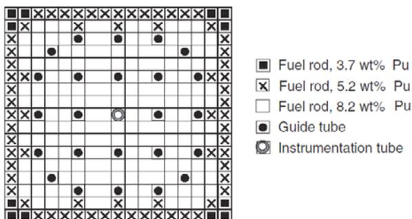
**Figure 1:** PWR MOX assembly design of the 17x17—24 type with assembly averaged plutonium concentration of 7.2 wt% Pu. (From [10])
