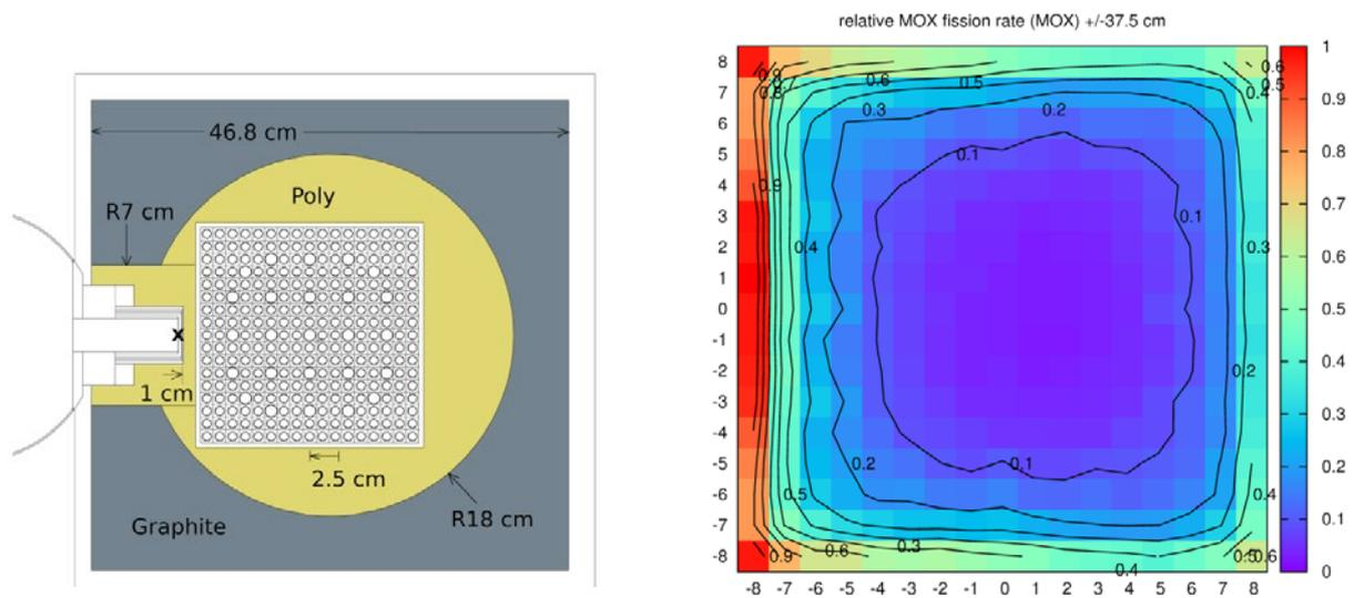
**Figure 3:** Left: Cross-section of the HGETv1a instrument geometry including a D-T generator (far left, with neutrons generated at the location of the x), a PWR assembly, and a combination of poly and graphite moderator/reflector. Right: Mapping of fission rate induced by low-energy neutrons, assuming the HGETv1a design (each pixel represents one fuel pin).
