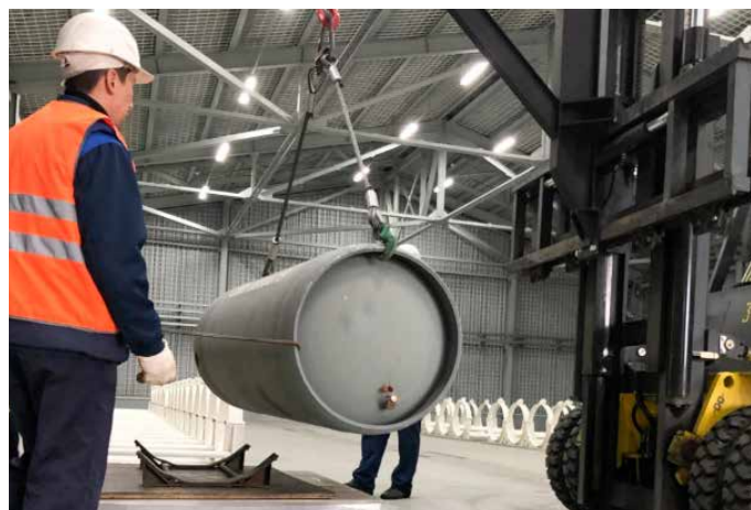
Figure 1: 30B uranium hexafluoride container at the IAEA Low Enriched Uranium Bank in Kazakhstan. Credit: IAEA, 2019.
