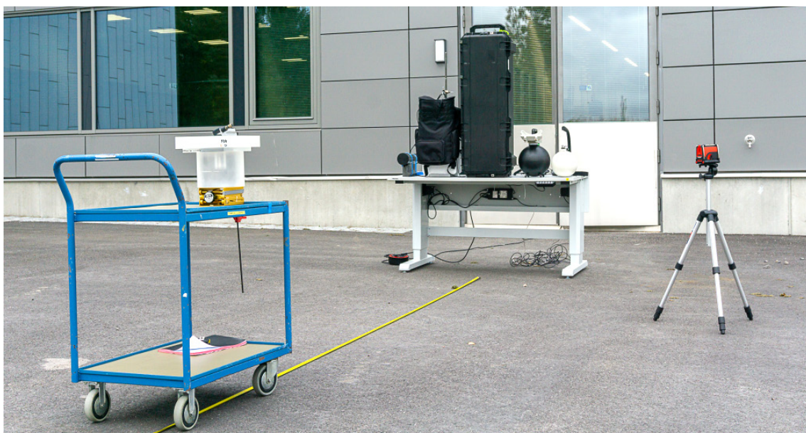
Figure 2: The setup depicting outdoor measurements. Moderated ^{252}\text{Cf} source was placed on the table trolley and the source-to-detector distance was measured with a laser range finder.
