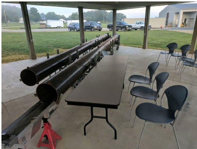
Figure 5: Setup of the piping for testing of battery. The cart ran until the end of the pipe, then reversed to the point of origin, summing up total distance.
