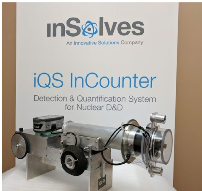
Figure 1: The InCounter cart resting on a stand. From right to left, the camera, lights, LIDAR, detector and surrounding detector housing, and cart chassis.
