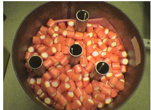
- Figure 4 - Vinyl matrix used for the FUNE calibration
