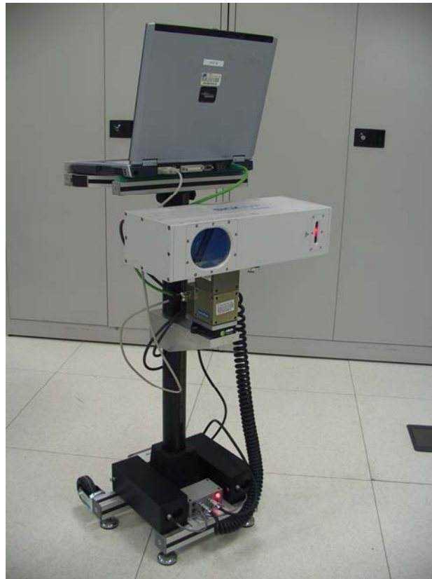
Figure 8: Instrument for scanning the container surfaces.
