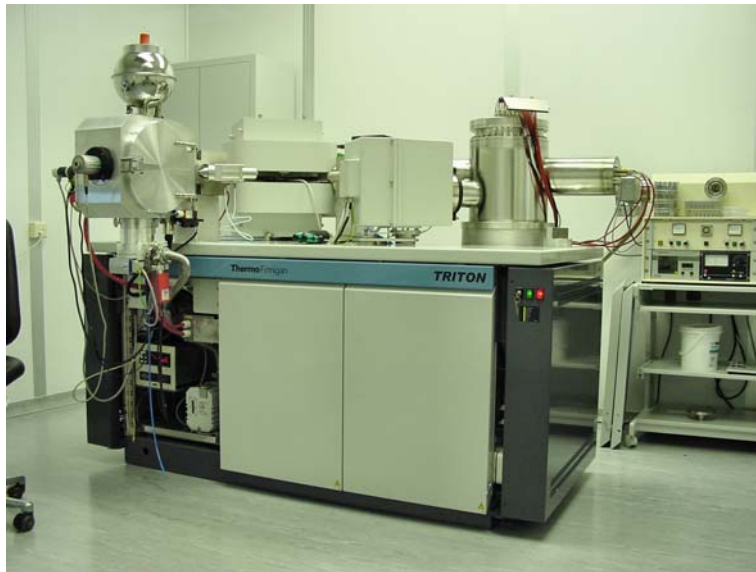
Figure 2. Thermal ionization mass spectrometer at SAL for bulk analysis.
