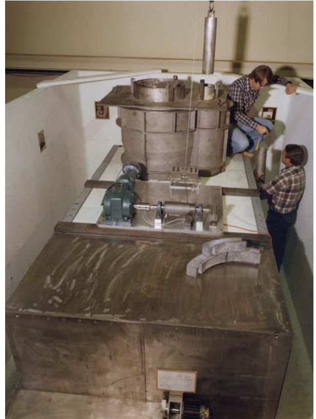
Fig. 1. The spent naval fuel shuffler is depicted above. A container is suspended above a small tube where assays are done on waste material inside the container. A larger tube, to the left, is for fuel assemblies.
