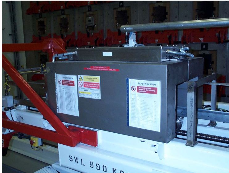
Fig 3: Neutron coincidence counter integrated into magazine handler (from ref 11)
