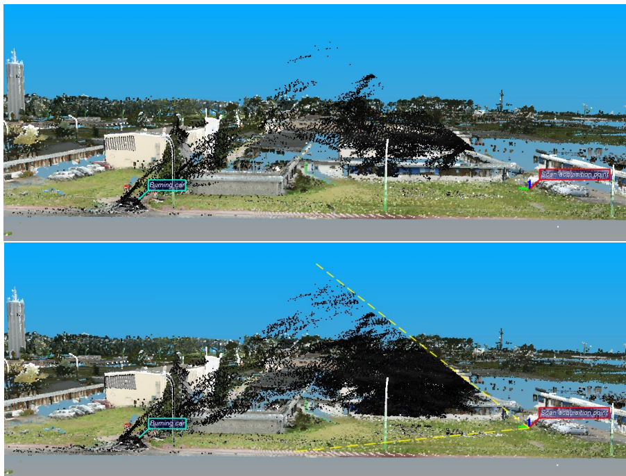
Figure 7: Two snapshots of the 3D model of the smoke plumes emanating from the burning car on the left. The laser scanner is located at the right. The dashed lines indicate the scanning field of view (FoV). Only the smoke plumes inside the FoV were captured.
