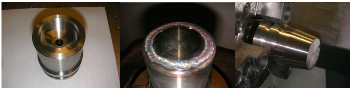
Photo 6: Rough body of a seal (left), welded identity of top a rough seal (center) and final machining of the seal (right)
