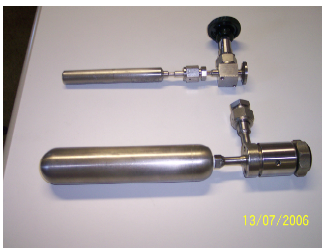
Figure 5 Ampoules 1S and 3S used to store isotope reference materials MRI 2.5
