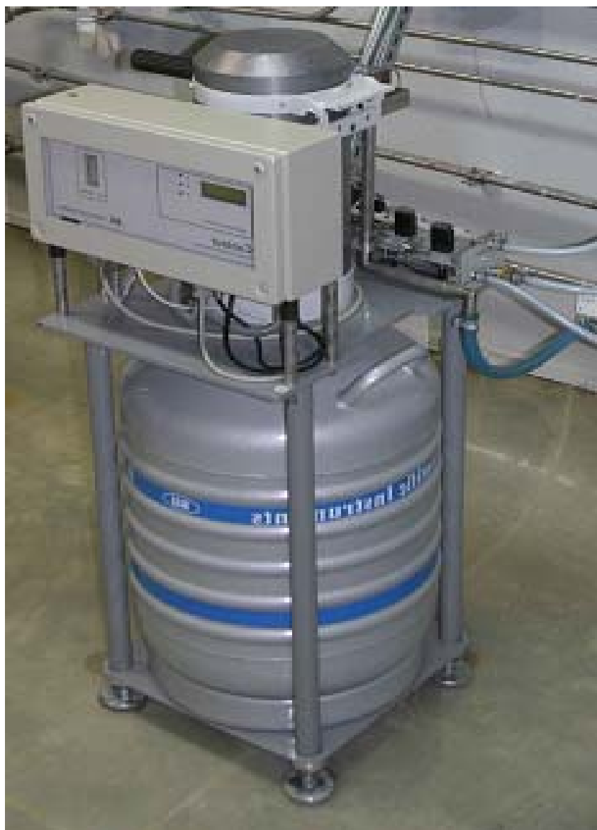
Fig.2. The external view of the automated HPGe spectrometer
