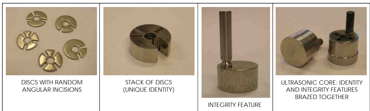
Photo 1 : Core of ultrasonic seals.
