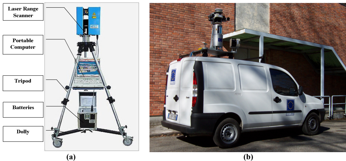
Figure 1: (a) Laser scanner on tripod with dolly for indoor operation; (b) Laser scanner mounted on vehicle for outdoor operation.
