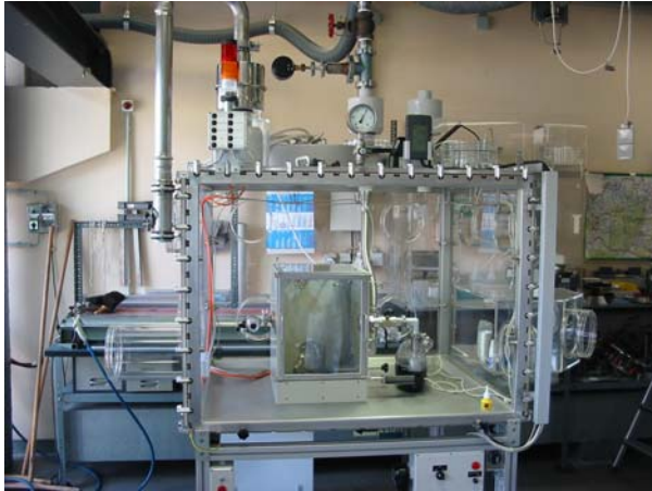
Figure 1 Dedicated glove-box for taking fingerprints from contaminated items.
