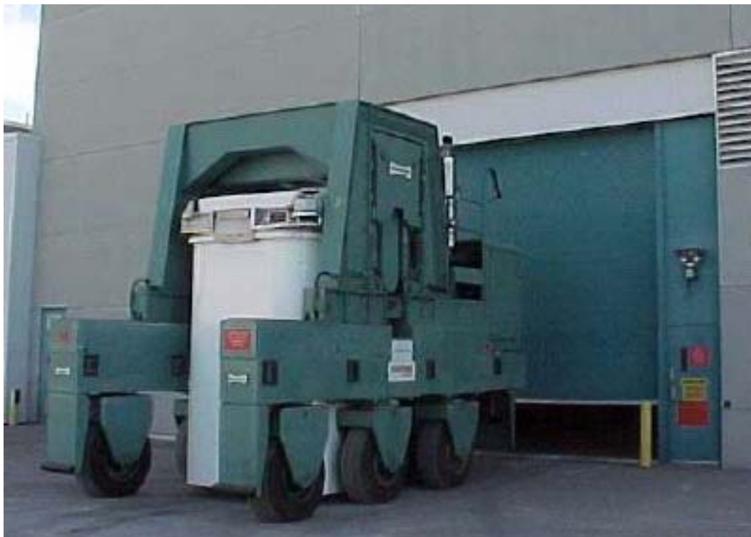
Figure 2 - A loaded DSC being transported
