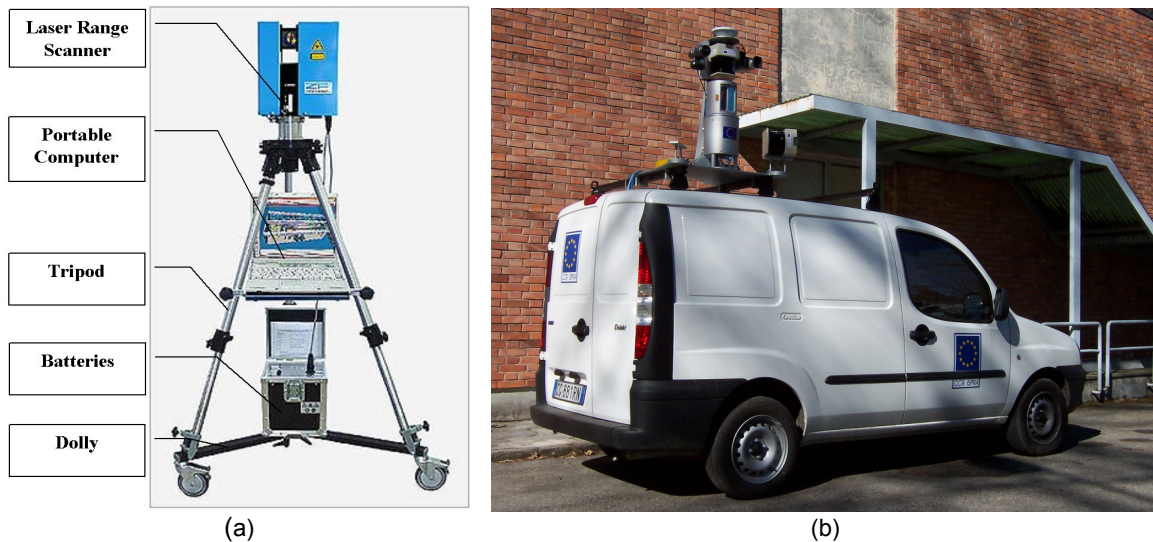
Figure 2: (a) Laser scanner on tripod with dolly for indoor operation (b) Laser scanner mounted on vehicle for outdoor operation.
