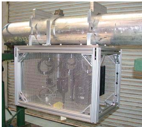
Fig. 6: Typical configuration with the monitor connected to the UF 6 pipe. The cage with instrumentation is connected to the pipe by the end brackets; the middle bracket carries the source.
