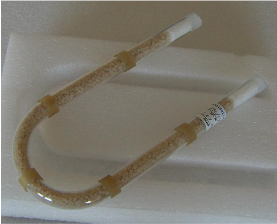
Fig. 3. Special calibration source of the spectrometer
