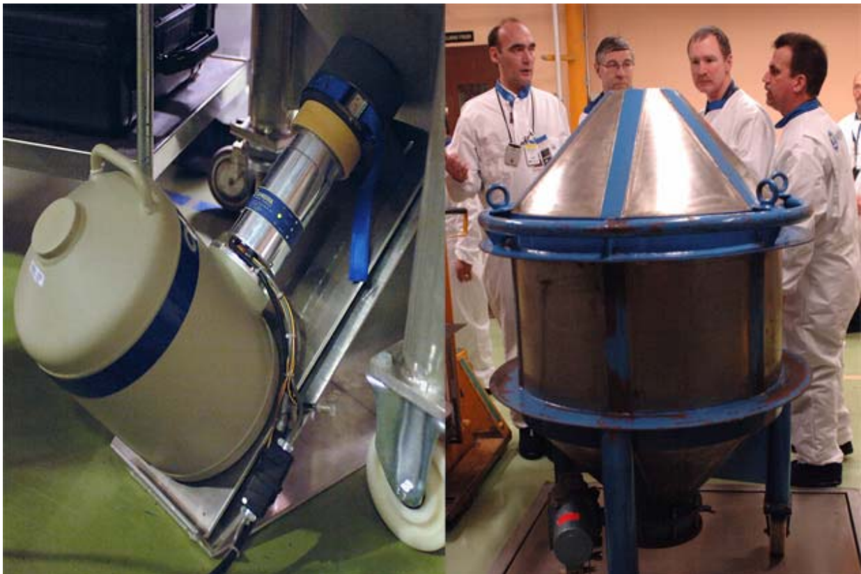
Measuring uranium powder in a "hopper" with a germanium detector
