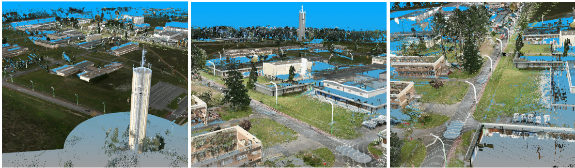
Figure 5: Partial 3D Overview of the CESTA site. Eight laser scans were used to create this model. Each model point has an accuracy of about 2cm. Processing time amounted to about 3 hours.
