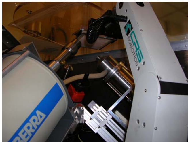
Figure 1. Inside view of XRF screening device showing robotic arm holding a swipe sample above the X-ray tube (right side) and Si(Li) detector with preliminary energy selection filter.
