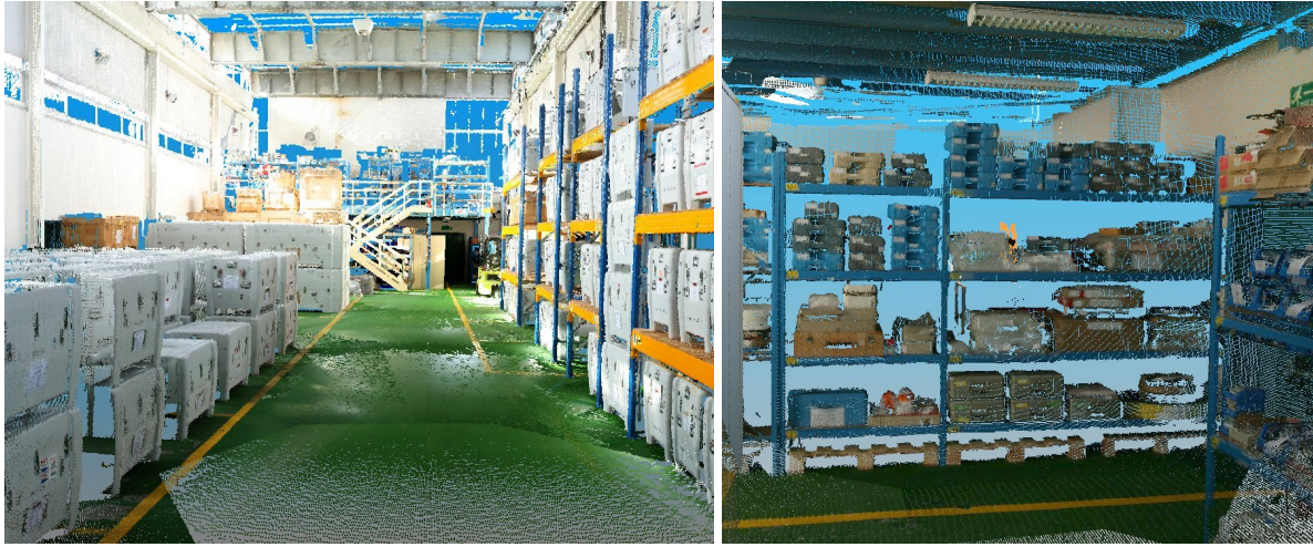
Figure 3: View of the 3D reconstructed model of a warehouse. Ten laser scans were used to build this model, taking approximately 60 minutes. All points were measured with an accuracy of 4mm. Light blue indicates areas for which no 3D information is available (i.e., have not been scanned).
