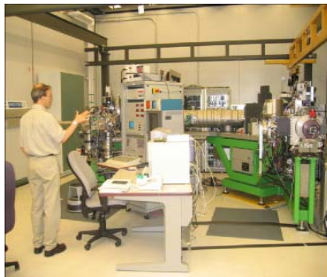
Figure 3. Cameca 1280 Ultra-High sensitivity SIMS instrument.
