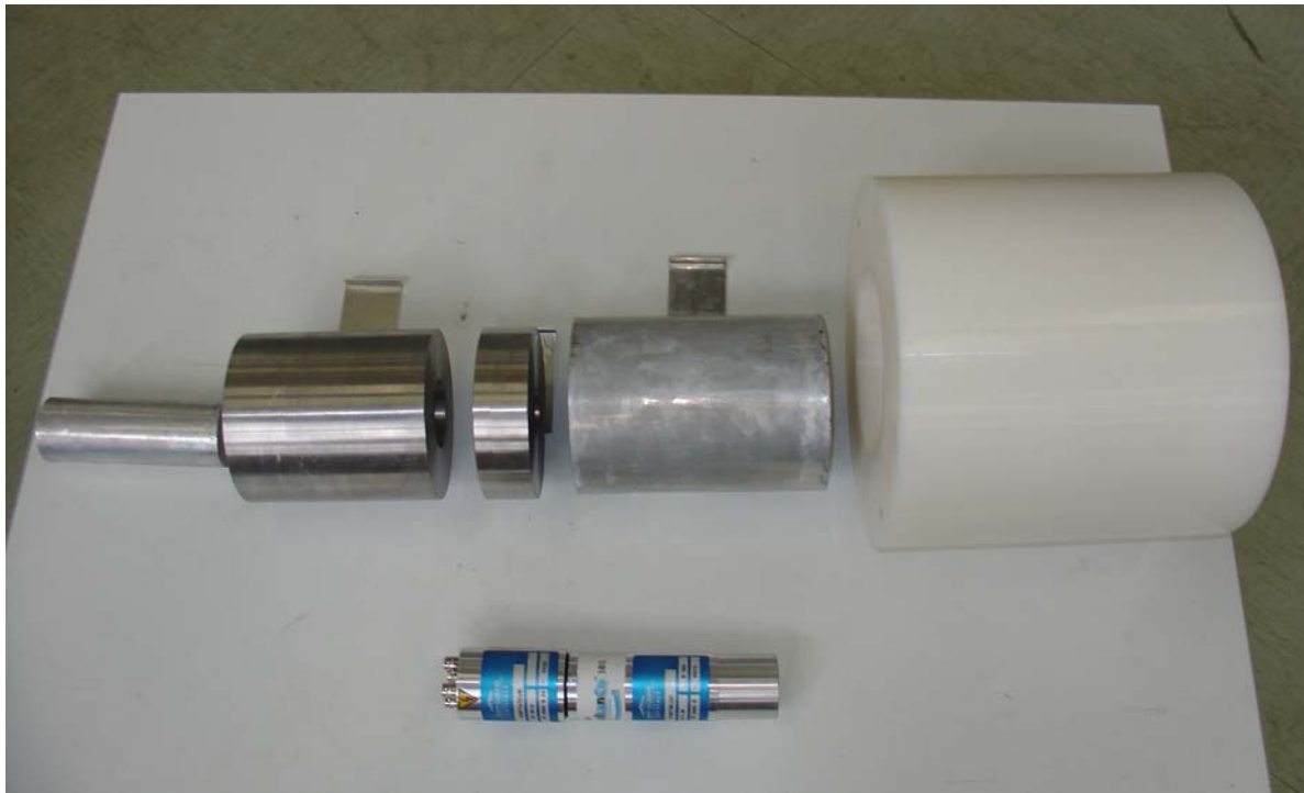
Figure 5: Shielding components: (from left) cadmium cup, two tungsten cylinders, further cadmium cup and polyethylene cylinder. The LaBr 3 :Ce scintillation detector is also shown.
