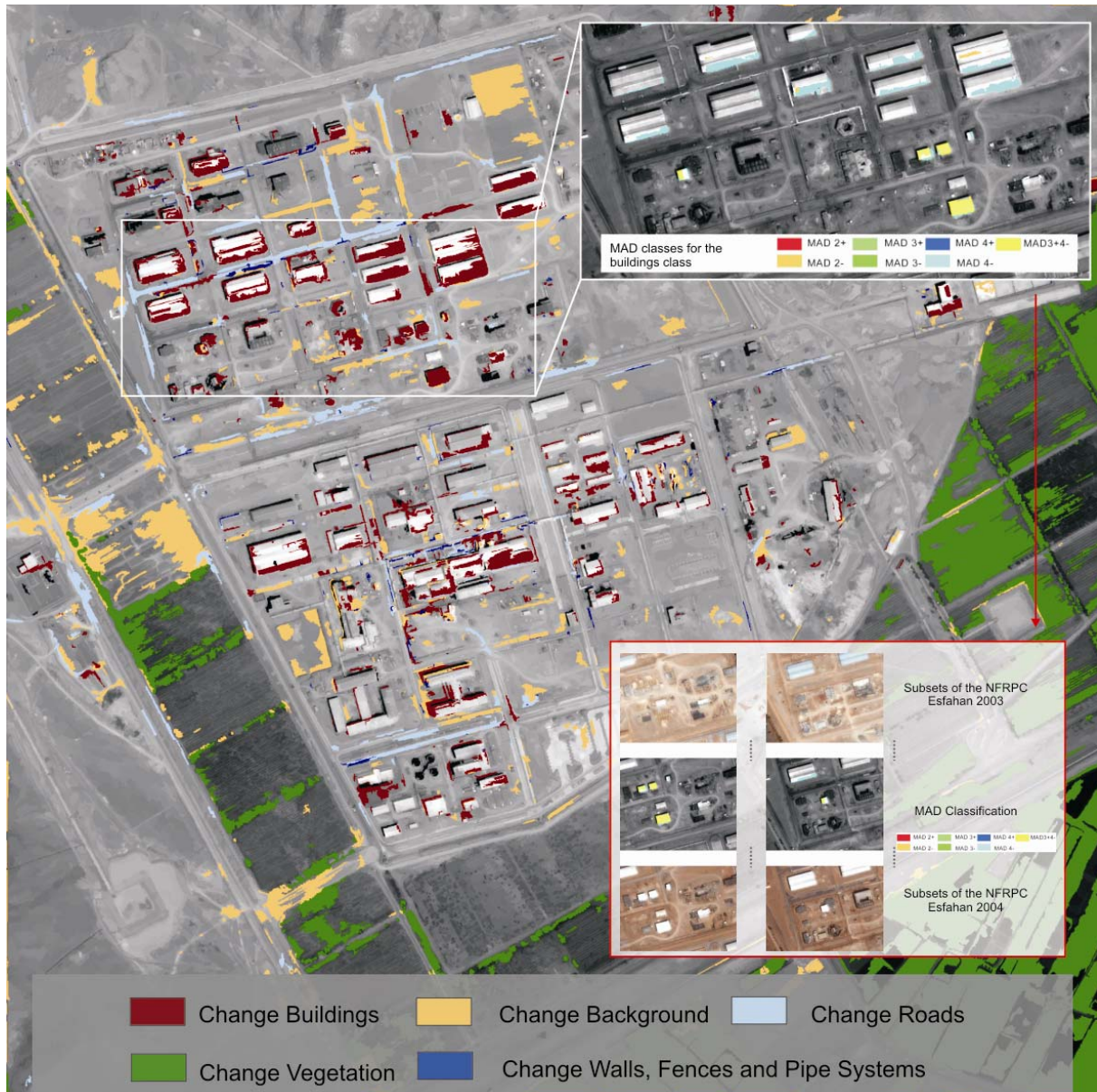
Figure 4: Comprehensive change detection result for the NFRPC Esfahan. The background image shows all significant changes in the time period 2003 to 2004. Within the white frame different kind of changes are discriminated. The red frame shows the detect new constructed buildings and a comparison between 2003 and 2004.
