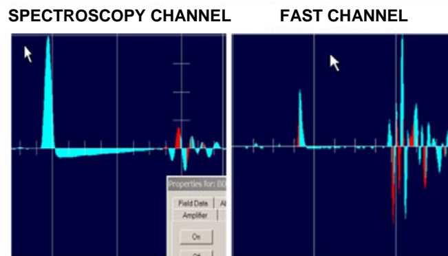
Fig. 8: Amplitude relationships between signal and noise pulses in the slow and fast channels of the MCA.
