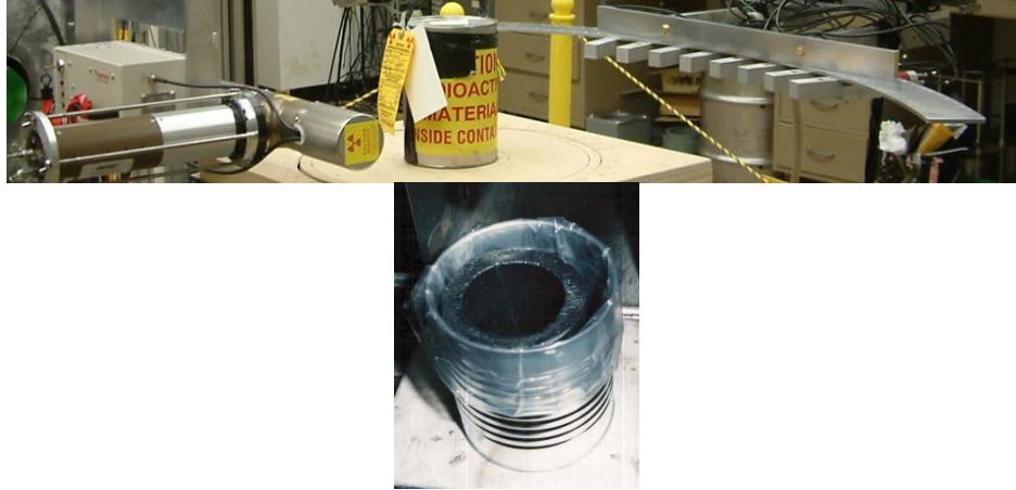
Figure 3: Source-uranium metal-casting-detector configuration for imaging
