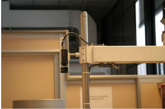
Figure 6: Camera mounted on the tool flange
