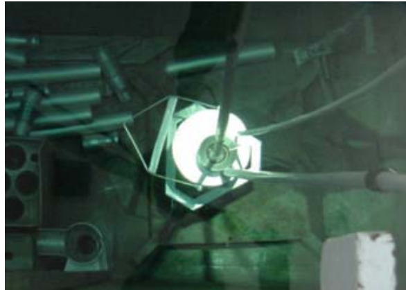
Figure 5. Photo of the AEFC on the bottom of the HIFAR spent fuel pool. The flexible tube to the surface contains the electronics cables and the ridged PVC tube contains the AmLi neutron source transfer cable.
