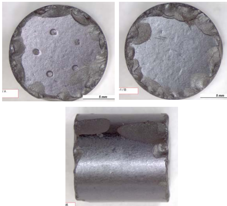
Figure 2 Pellet seized in Hungary and analysed at ITU. This pellet shows markings at the bottom and a slight dishing at the opposite side of the pellet.
