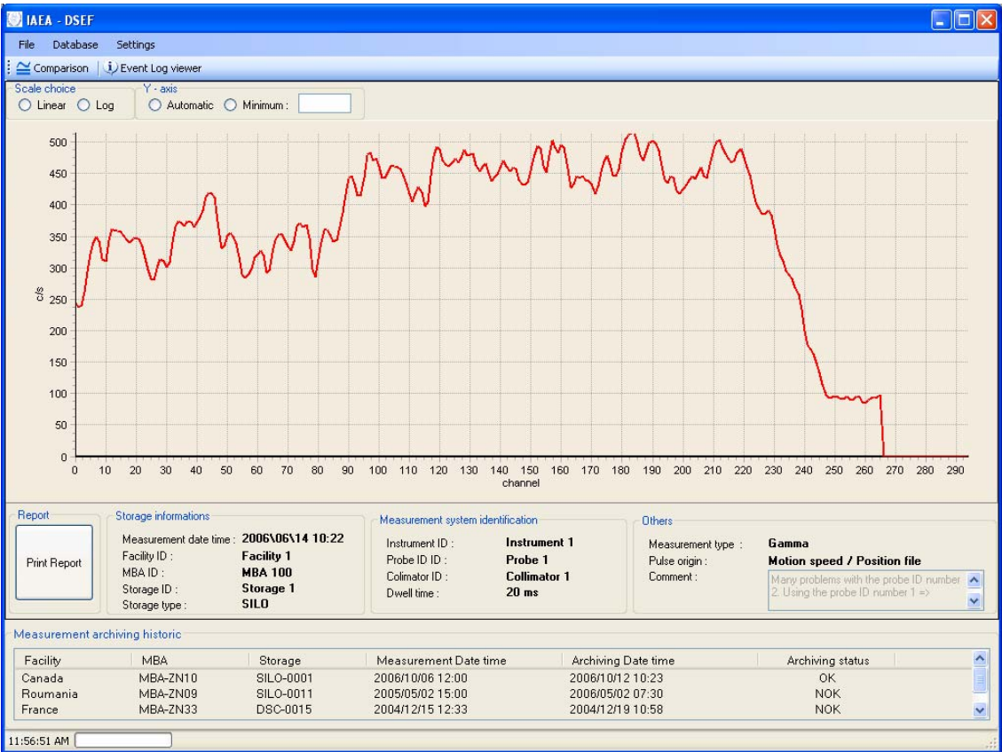
Figure 10 a) : Display of a spectrum store in one of the interpreted format.
