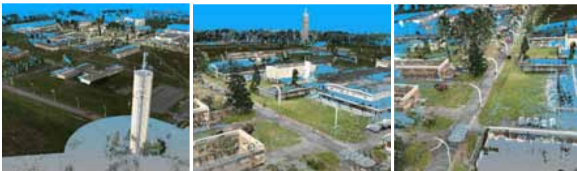
Figure 5: Partial 3D Overview of the CESTA site. Eight laser scans were used to create this model. Each model point has an accuracy of about 2cm. Processing time amounted to about 3 hours.
