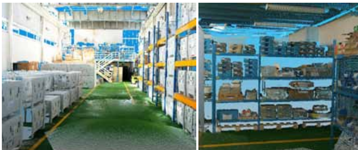
Figure 3: View of the 3D reconstructed model of a warehouse. Ten laser scans were used to build this model, taking approximately 60 minutes. All points were measured with an accuracy of 4mm. Light blue indicates areas for which no 3D information is available (i.e., have not been scanned).
