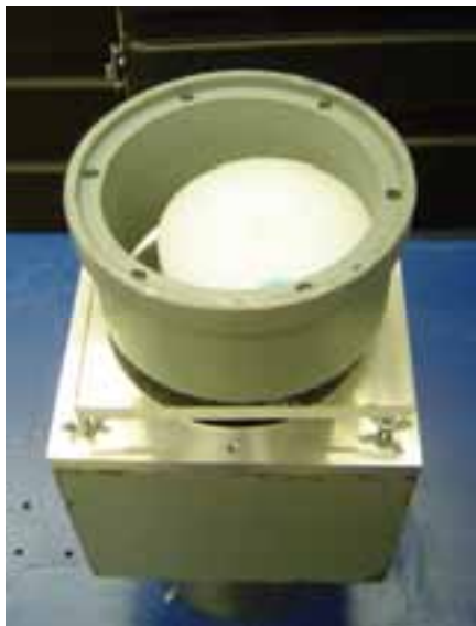
Figure 8: 3D object of lead, aluminum, polyethylene, and Plexiglas.
