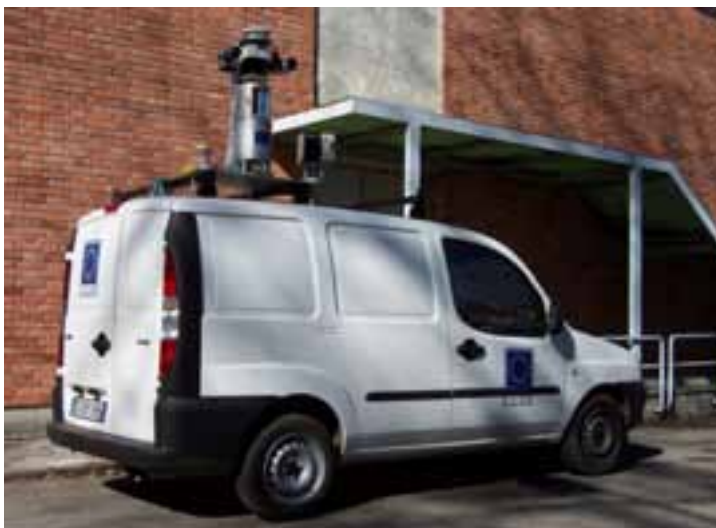
Figure 1: (left) Laser scanner on tripod with dolly for indoor operation; (right) Laser scanner mounted on vehicle for outdoor operation.
