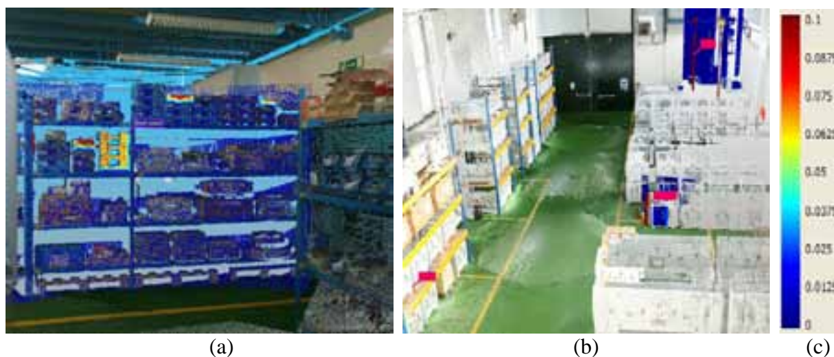
Figure 4: Detection of changes inside the warehouse. Changes are indicated in red/orange: (a) changes in the shelves area; (b) changes in warehouse’s main hall – three objects were detected: a mobile phone on the shelf (bottom left), the crane cable (top right) and the forklift (centre-right); (c) false colour code – red corresponds to distance changes larger than 10cm; change in the object in (a) is about 6.5cm.
