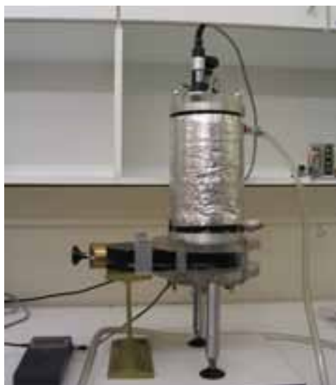
Figure 1: Aerosol deposition chamber designed at the IRMM for the preparation of \text{UO}_2\text{F}_2 particles from the controlled hydrolysis of \text{UF}_6 .
