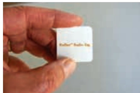
Figure 1: A RuBee Radio Tag (4 bit CPU, 1kB sRam, and lithium battery with expected life of 5 years).
