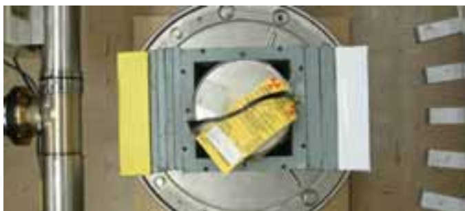
Figure 6: DU casting within a 1-in.-thick lead box surrounding and 4-in. thickness of lead plates in front and back.
