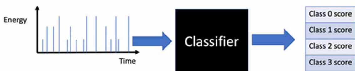
Figure 2: List-Mode Linear Classifier Architecture
