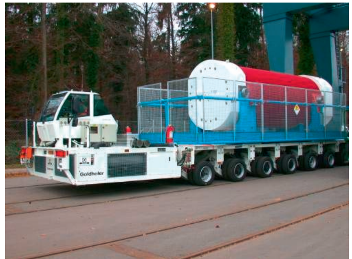
Figure 8: Castor® cask with shock absorbers at both ends.
