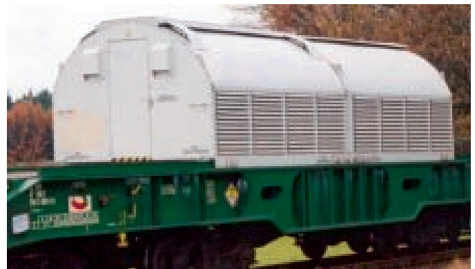
Figure 7: Cask covered by protective coachwork during transport.
