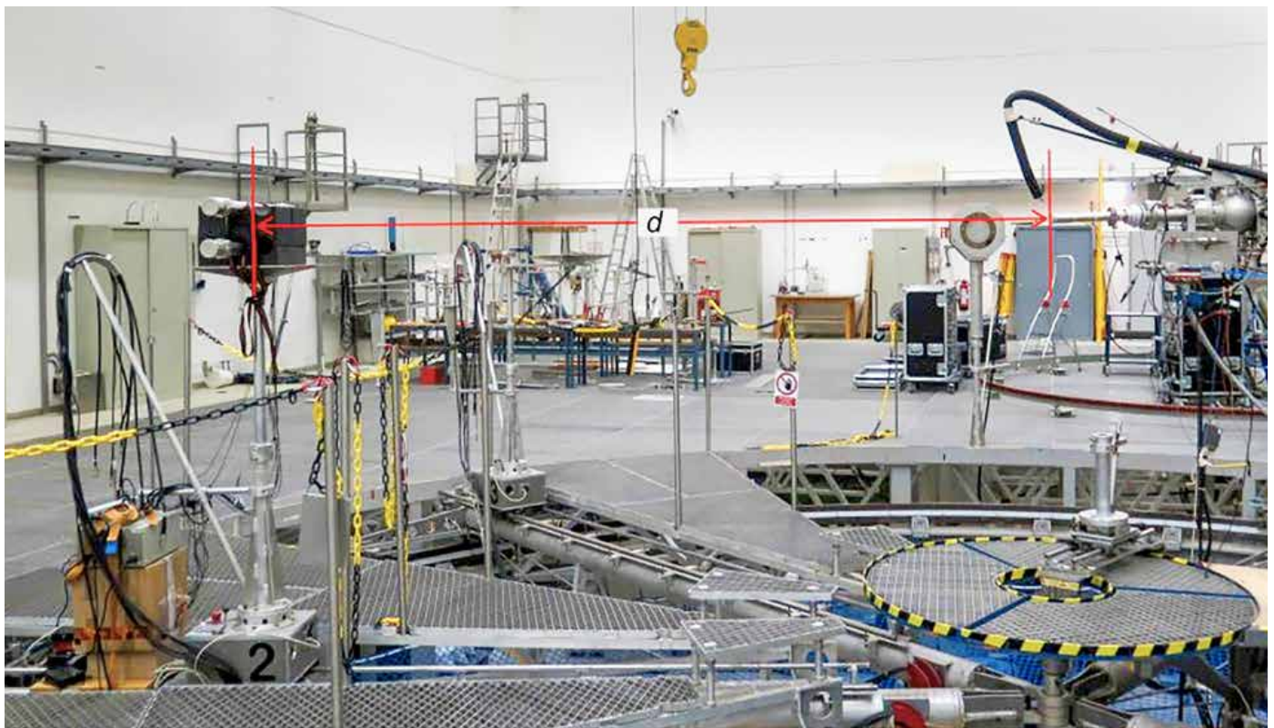
Figure 4: Picture of the experimental set-up in the low-scattering measurement hall at PTB. Target-to-detector distance is indicated by the red line.
