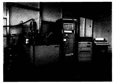
Fig. 1. Transportable quadrupole mass spectrometer for  $\mathsf{UF}_6$  isotopic analyses used by DCS Luxembourg
