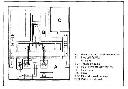
Figure 1. Pilot conditioning facility. Layout of 4.5 m level. Nuclear Material Flow, Process of LWR Spent Fuel
