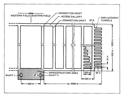
Figure 2. Schematic view of emplacement floor
