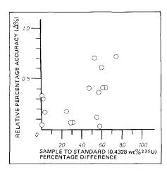
Fig. 4. Distribution of the accuracy against sample to standard relative difference for the 0.4328 wt% reference sample
