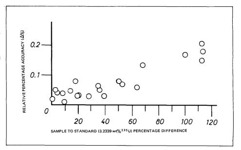
Fig. 3. Behaviour of the accuracy against sample to standard relative difference for the 3.2339 wt% enriched reference sample
