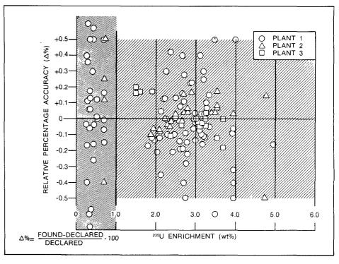
Fig. 2. Typical differences between declared and measured values obtained in three different enrichment plants
