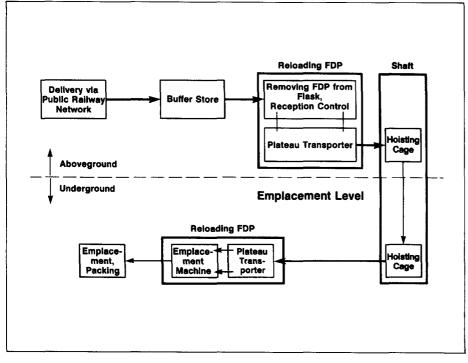
Figure 3. Material flow diagram
