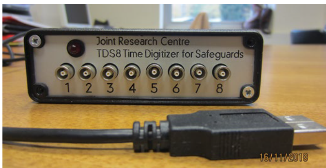
Figure 1: The TDS8 and TDS32 list-mode devices developed at JRC, one with 8 front panel inputs, the other with 32.
