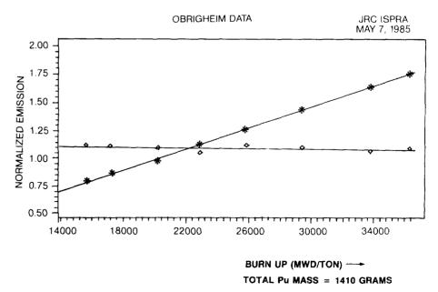
Fig. 11 - Plutonium emission analysis: normalized passive and active emissions as functions of ournup
