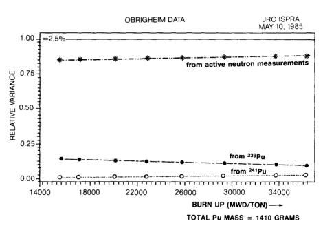
Fig. 7 - Active assay: plutonium error propagation analysis
