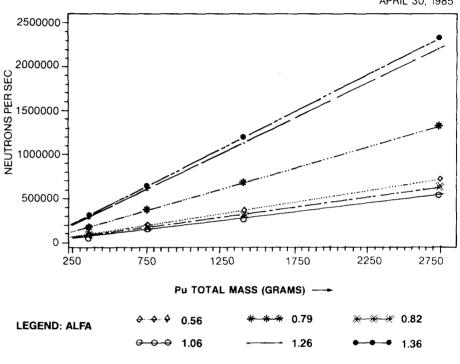
Fig. 10 - Pu passive emission at different isotopic compositions vs Pu mass
