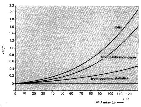
Fig. 5 - PHONID error structure with 400 sec counting time
