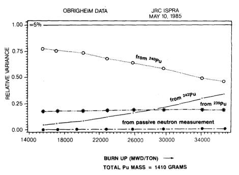
Fig. 6 - Passive assay: plutonium error propagation analysis
