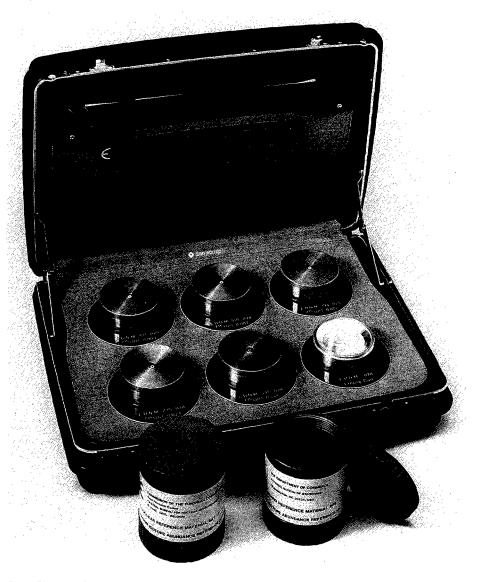
The NRM 171 / SRM 969 in its case, together with two transport containers for the single standard samples. The set is completed with an empty can, which allows comparison measurements on material with an unknown enrichment in exactly the same geometrical conditions.
