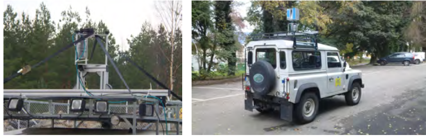
Figure 3. Hybrid setup for the MLSP in the 2014 verification. (left) detail of the mobile laser mounting on top of the car. (right) full hybrid system used during the verification.
