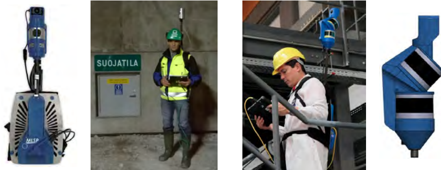
Figure 4. MLSP systems used for the verifications. (left) single-head backpack with one Velodyne HDL-32E laser sensor, demonstrated in the 2014 verification and used in the 2015 and 2017 verifications. (right) dual-head backpack with two Velodyne VLP-16 sensors configured in a tilted position, used from the 2019 verification.
