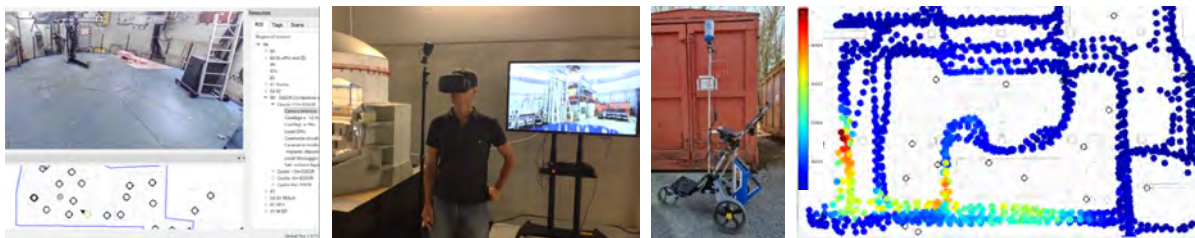
Figure 13. Other applications. From left to right: (1) decommissioning 3D database (3DIMS), (2) VR visualization tool, (3) radiation mapping device with the MLSP and (4) radiation mapping results in 3DIMS.
