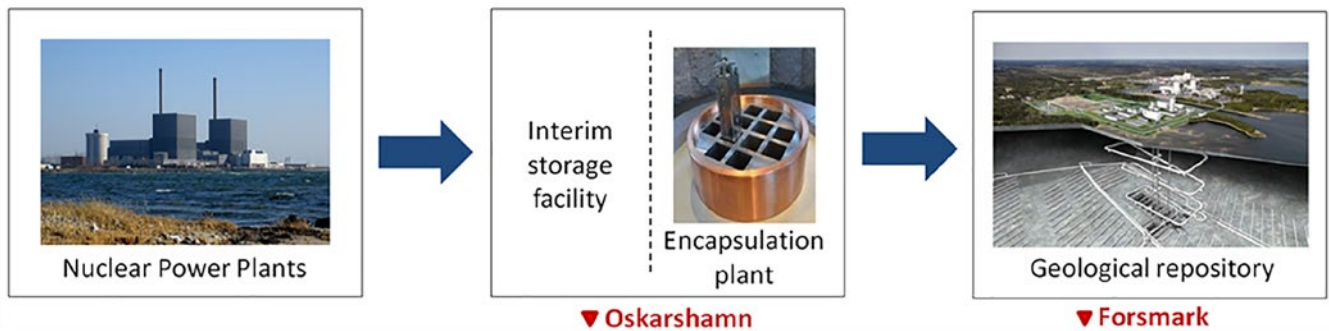
Figure 1. The spent fuel transfers in the Swedish system for final disposal of spent nuclear fuel.
