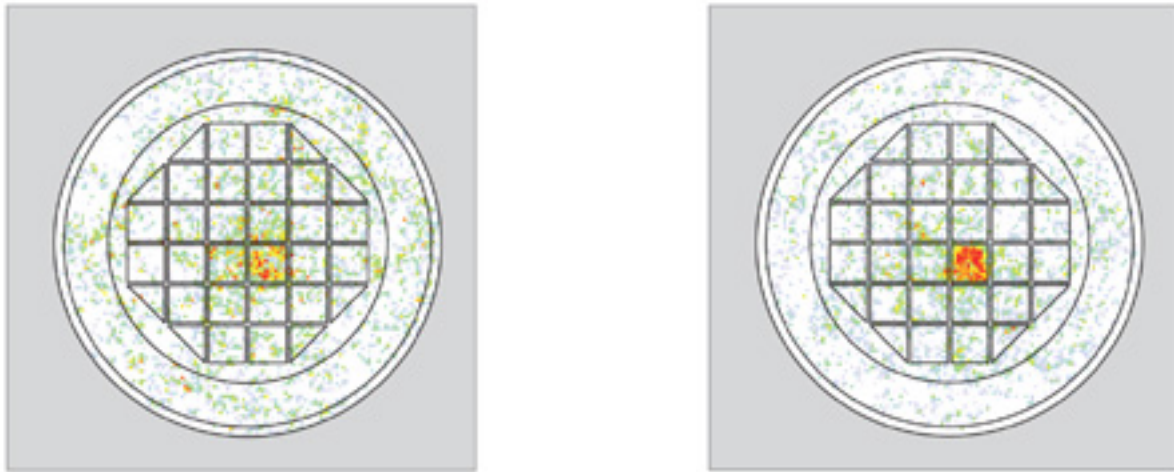
Figure 3: Top-view of the reconstructed CASTOR® density, averaged over vertical axis, obtained using absorbed muon (left) and passing-through muon information (right). The simulated container has one missing bar. Both images are the difference between the images obtained from the CASTOR under examination and reference images, obtained analysing a container without missing bars. The container structure including the bar grid is added for reference.
