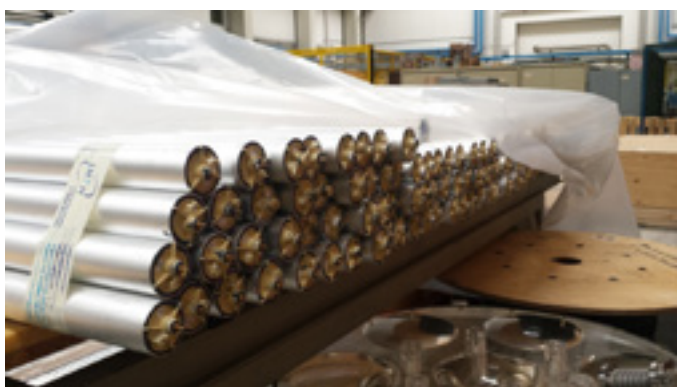
Figure 5: Set of 2m long drift tubes produced in LNL INFN laboratory.
