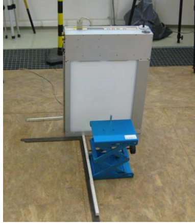
Figure 1: Picture of the experimental setup used in the measurements. The Fission Meter is placed on an open mesh flooring which is covered by plywood. It is used in its closed configuration and the white moderator side is facing outwards. The source is placed on the edge of a scissor lift and positioned in the center of the Fission Meter. All walls, ceiling and the concrete floor under the open mesh flooring are more than 2 m away from the source and the detector in order to reduce scattering.
