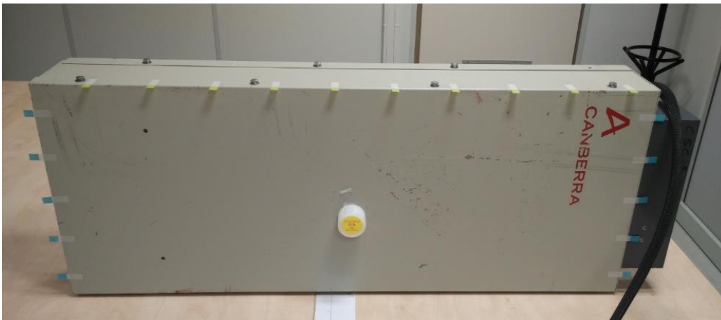
Figure 2: Picture of the Canberra WM3400 neutron coincidence counter and position of the ^{252}\text{Cf} source used in the testing.
