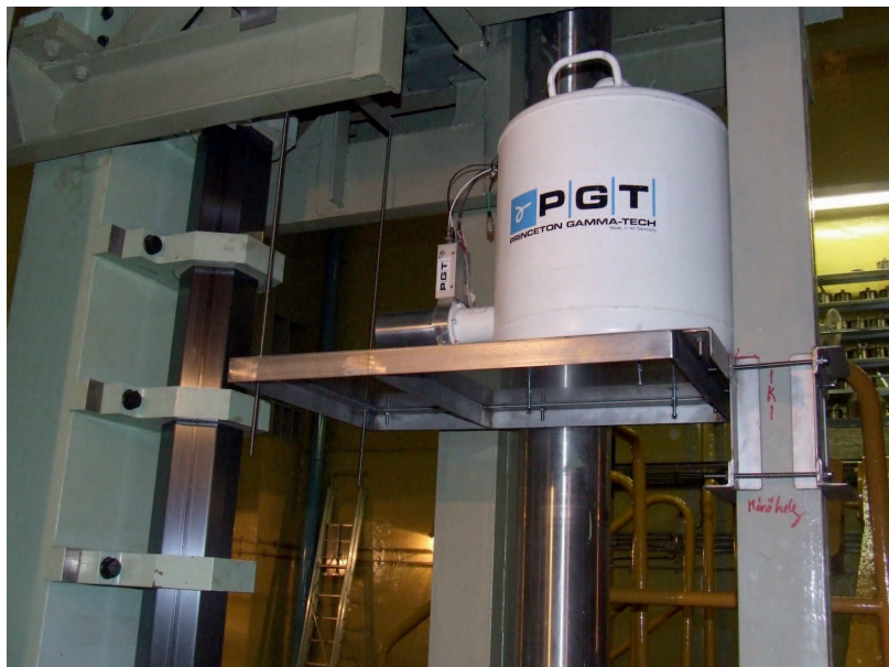
Fig. 1: HPGe Detector stand and assembly in measuring position
