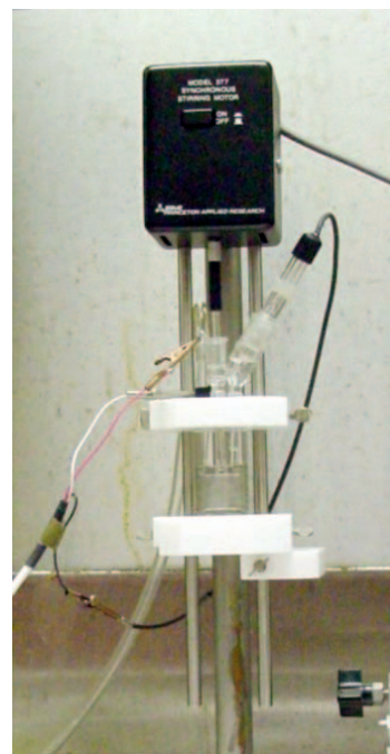
Fig 2: Cell Assembly, SRNL design, with modified PAR stirring motor
