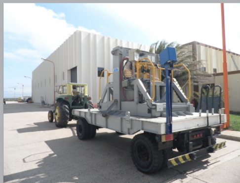
Unattended Monitoring of Spent Fuel Transfers using the Mobile Unattended Neutron Detector (MUND) at a power reactor in Argentina
