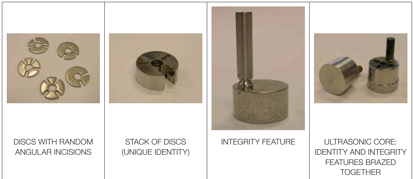
Photo 1: Core of ultrasonic seals.
