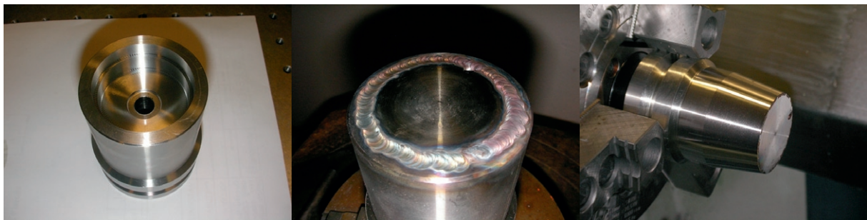
Photo 10: Rough body of a seal (left), welded identity of top a rough seal (center) and final machining of the seal (right).
