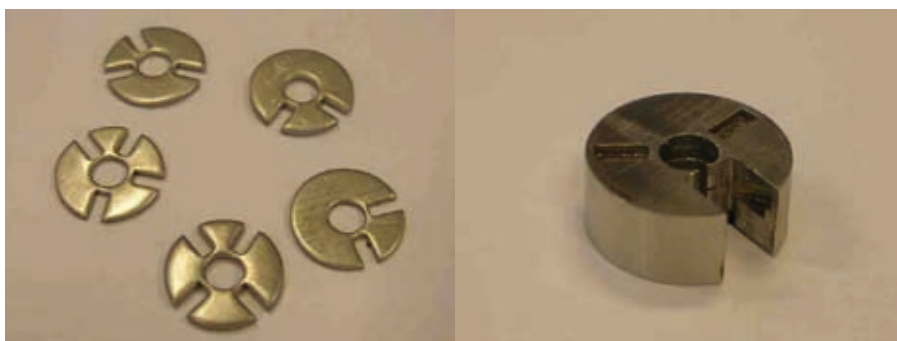
Fig. 2: Discs used for the identity and brazed together
