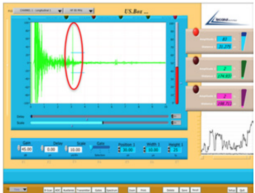
Figure 6: Set-up of the ultrasonic investigation and corresponding A-scan acquisition.
