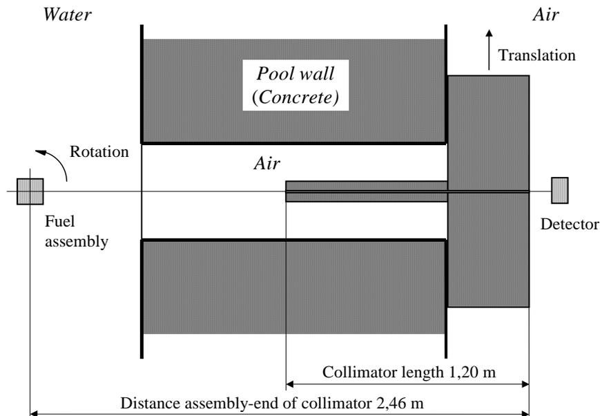
Fig. 1: Pool-side equipment. Schematic view from above.
