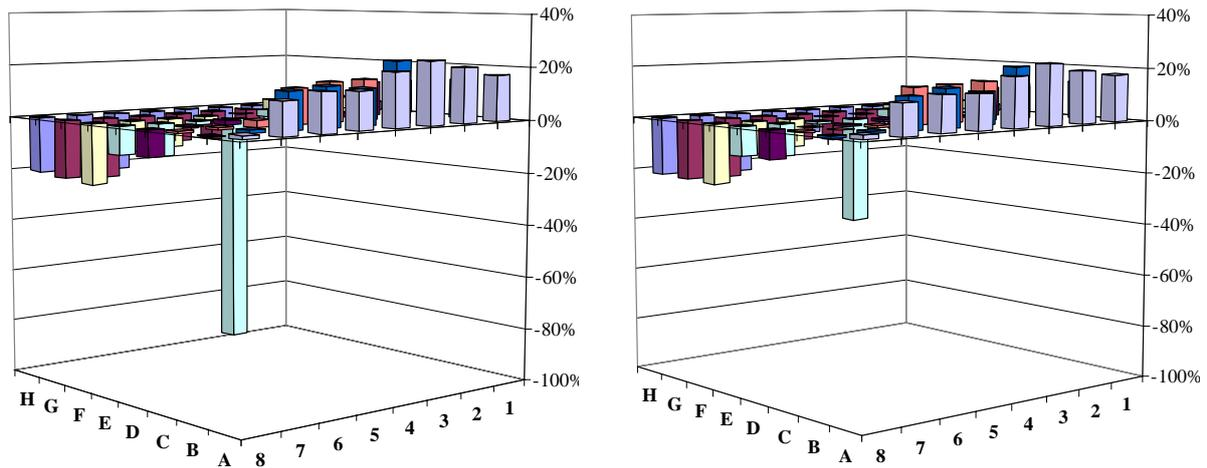
**Fig. 7:** Obtained deviations from the average activity in measurements using the laboratory equipment. In the left figure, rod (E,5) had been replaced with a non-active rod. In the right figure, rod (E,5) had been removed without replacement. In both cases, the value in that position is significantly smaller than the other rods. The distribution of activities in the other positions reflects the actual distribution, measured with 1.5 % accuracy ( $1 \sigma$ ).
