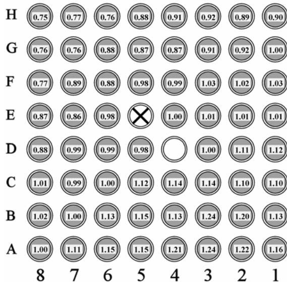
**Fig. 5:** The activity configuration in the laboratory model of a fuel assembly of the ABB 8x8 BWR type. The activities are normalised to a mean value of unity. Position (D,4) normally contains a water channel, which was modelled using an empty rod. The ability to detect rod removal or replacement at position (E,5) was investigated. Replacement was modelled using a non-active rod.
