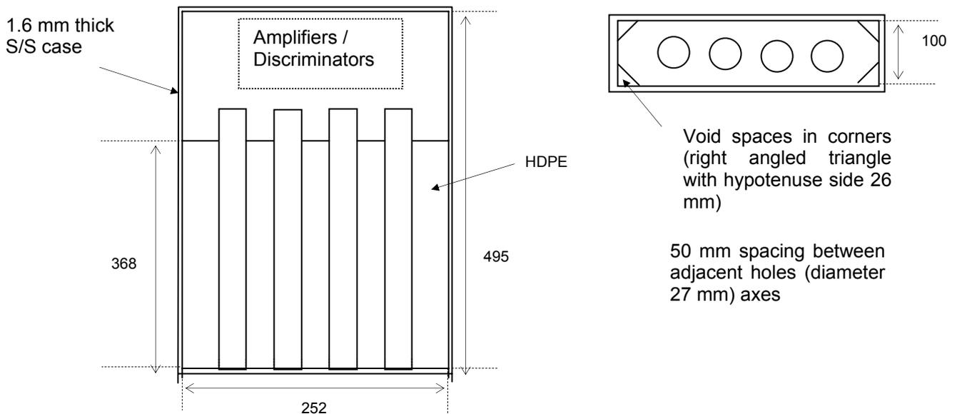
Figure 1. N50 configuration. Dimensions are given in mm.
