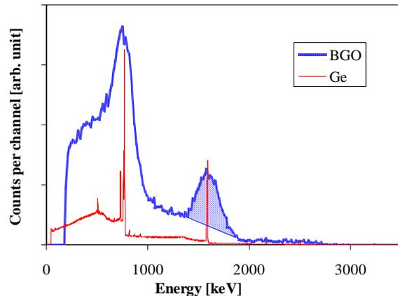
**Fig. 9:** A gamma-ray spectrum collected using a BGO detector and a 60 % efficiency Germanium detector. The cooling time of the assembly was four and six weeks, respectively. The peak analysis of the 1596-keV Ba-140 peak in the BGO spectrum is schematically illustrated.
