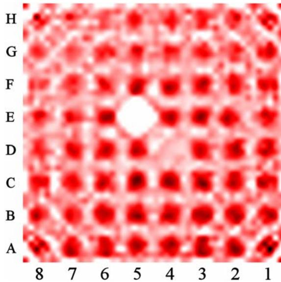
**Fig. 6.** Experimentally obtained image of the fuel model with a non-active rod in position (E,5) and an empty rod, representing the water channel, in position (D,4). The whole range of reconstructed activities is illustrated, where light areas illustrate low and dark areas illustrate high source concentration.
