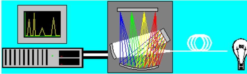
Figure 2.1: Light enters the spectrometer (middle gray object) through a slit and filter, reflects off of the collimating mirror, is diffracted by the grating, and reflects off the focusing mirror to the Silicon CCD detector array (taken from Ocean Optics). The object of interest would be illuminated by the light source using a split fiber cable (see reflection probe in Figure 2.2).
