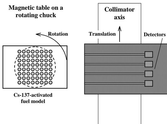
**Fig. 3:** Laboratory equipment. Schematic view from above.
