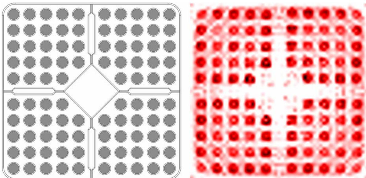
**Fig. 10:** The cross section of a SVEA-96S BWR fuel assembly (left) and an experimentally obtained image of the Ba-140 distribution (right). The whole range of reconstructed activities is covered. Light areas illustrate low and dark areas illustrate high source concentration.
