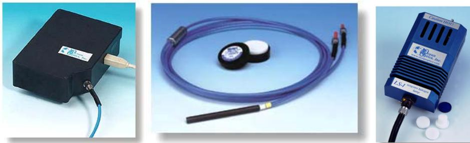
Figure 2.2: Ocean Optics HR2000 spectrometer with USB cable (square) and fiber optic cable (left); reflection probe and diffuse reflectance standard (center); tungsten halogen light source (right) (taken from Ocean Optics). The long metallic end of the reflection probe is used for sampling of the object, while the two red ends are connected to the light source and the spectrometer.
