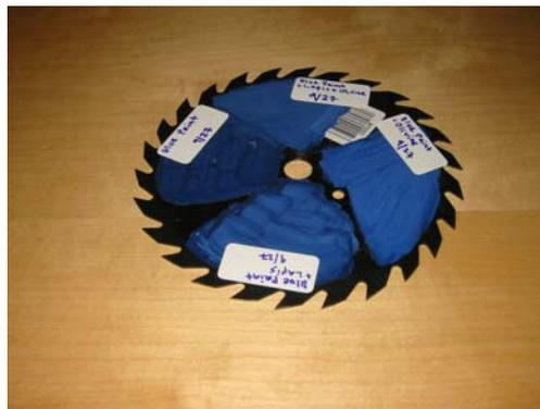
Figure 2.5: Blue paint samples on saw blade. Starting at bar code going clockwise: blue paint/olivine, blue paint/lapis, blue paint alone, and blue paint/lapis/olivine.
