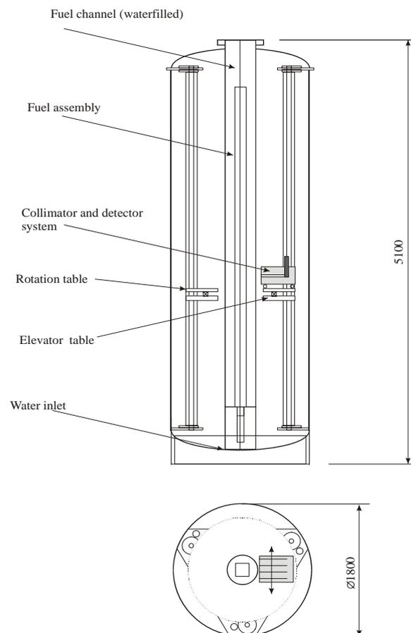
**Fig. 8:** Device for in-pool measurements. Schematic views from the side and from above.
