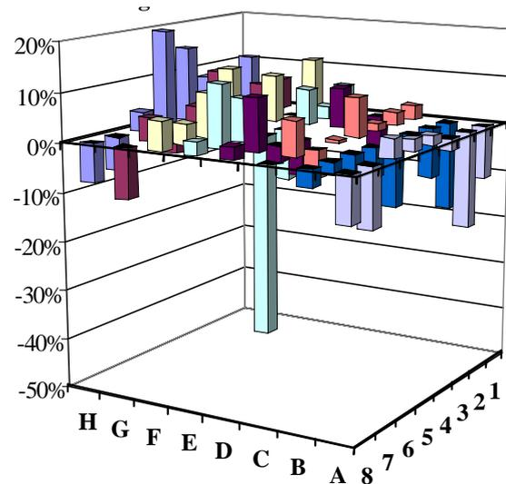
**Fig. 2:** The reconstructed rod activities experimentally obtained using the 1274 keV Eu-154 gamma-ray energy. Deviations from the average activity are illustrated. Note the significantly deviating value in the position of the removed rod, (E,5).
