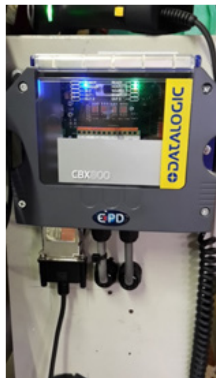
Figure 5: Datalogic CBX800 adapter that split the barcode scanner communication path
