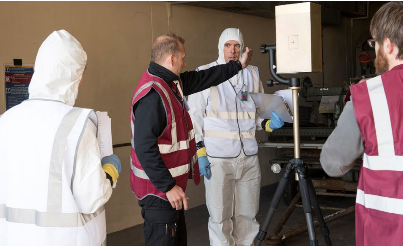
Figure 3: Radiation detection Equipment (RDE) is used to measure the local neutron count rate within a storage bunker that had been declared not to contain any B5 bombs as part of the absence verification procedure on a randomly selected location.
