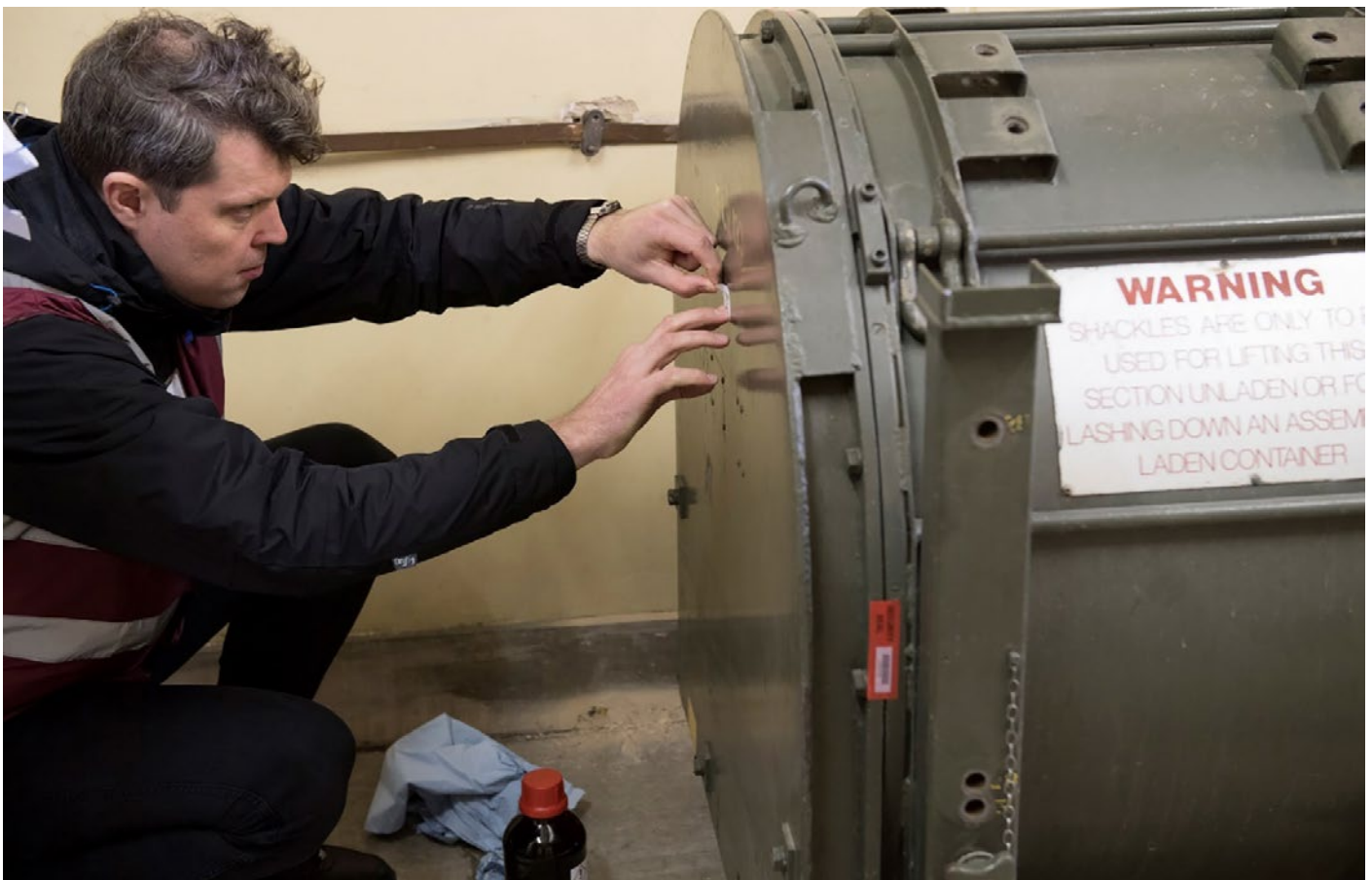
Figure 5: An applied Unique Identifier (UID) Tag is applied to the container of the B5 to ensure the individual item can be accounted for and tracked throughout the treaty lifetime.
