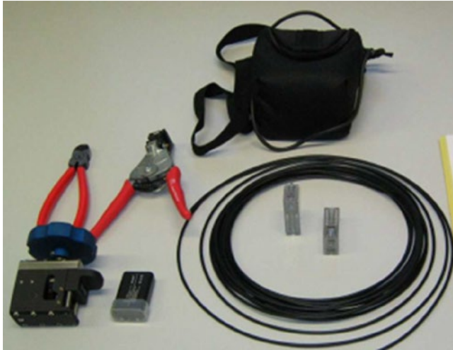
Figure 5: Equipment needed by the operator for applying the COBRA and the EOSS seal [9]
