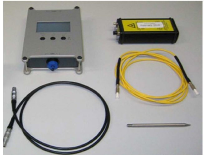
Figure 5: Equipment needed by the operator for applying the COBRA and the EOSS seal [9]
