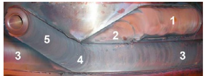
Figure 12. Welding tool rotation and sequences in the welding cycle: 1) acceleration sequence, 2) downward sequence, 3) joint line welding, 4) overlap sequence and 5) parking sequence.
