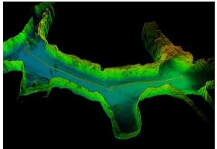
Figure 3: Map of underground mine created using LiDAR and a robot [25]
