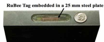
Figure 5: Embedded RuBee Tag inside steel plate
