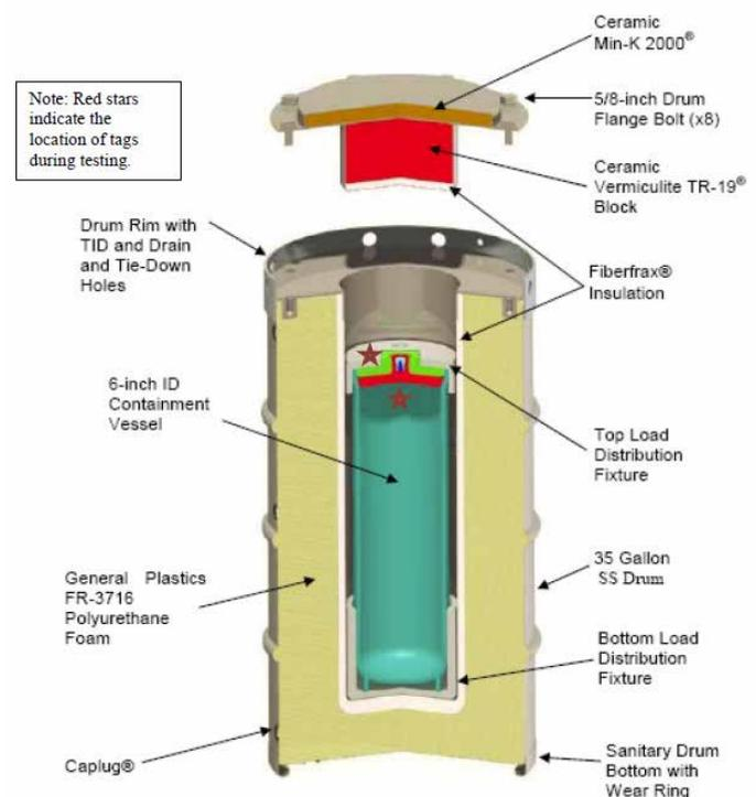
Figure 6: RuBee Tag inside US-DOE certified Type-B Model 9977 drum
