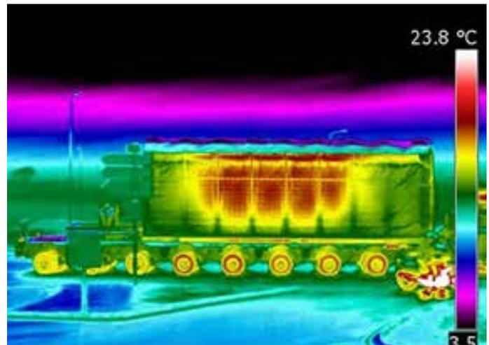
Figure 9: Thermal image of railcar CASTOR system [45]
