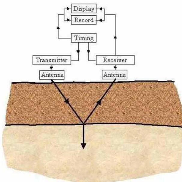
**Figure 7:** Working principle of GPR [36]
