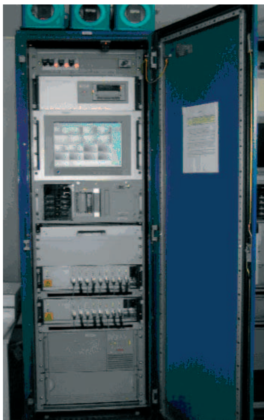
Figure 9: DMOS: Digital Multi-Camera Optical Surveillance (courtesy: IAEA, Vienna)
