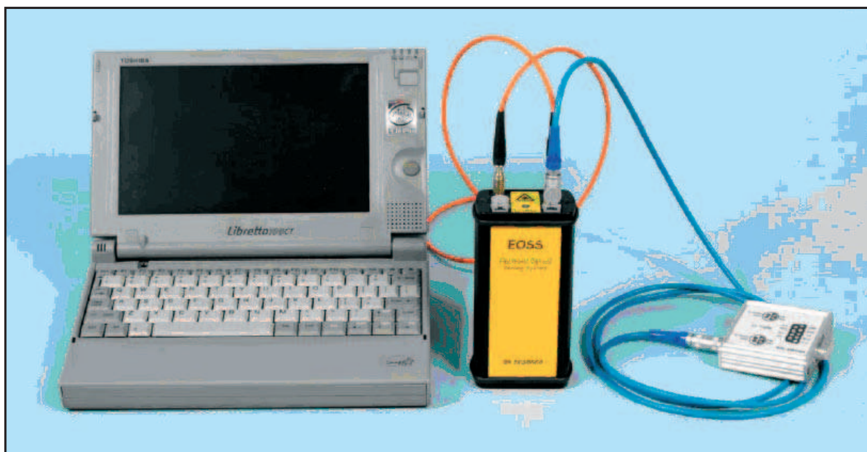
Figure 18: EOSS Seal (courtesy: IAEA, Vienna)
