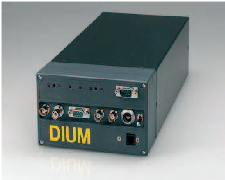
Figure 2: Digital Unattended Multi-channel Analyser prototype (courtesy: ICx Radiation GmbH)
