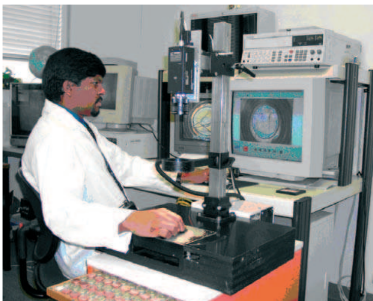
Figure 14: Comparison of metal cap seal images for seal validation (courtesy: IAEA, Vienna)
