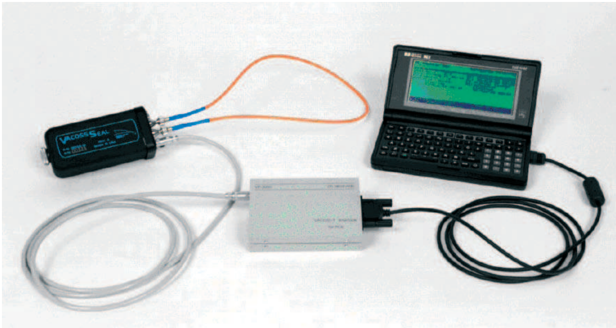
Figure 15: VACOSS 5.0 Electronic Seal with fibre optic loop, interface box and palmtop computer (courtesy: IAEA, Vienna)
