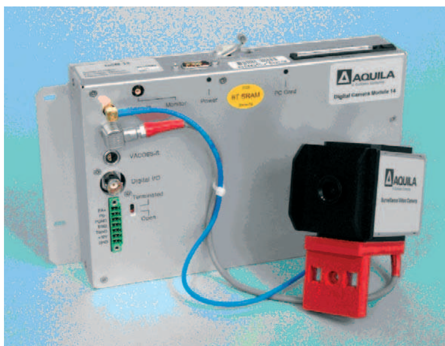
Figure 4: DCM 14 with video CCD camera (CCD: Charge Coupled Device) (courtesy: IAEA, Vienna)
