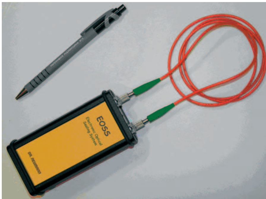
Figure 3: Electronic Optical Sealing System prototype (courtesy: Dr. Neumann Consultants)
