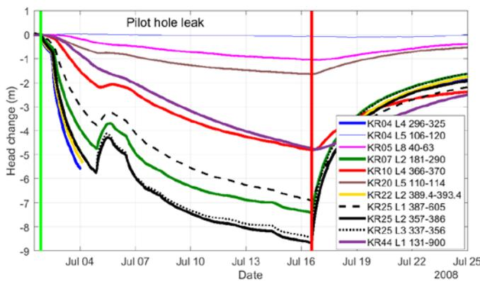
**Figure 5.** Change of hydraulic head in some monitored drillhole sections during a leak from a pilot hole intersecting the HZ20 structure. The vertical green and red lines mark the beginning and end of the leak, respectively. Drillhole section labels consist of a drillhole code (KR+number), section code (L+number), and range of drillhole length in metres.
