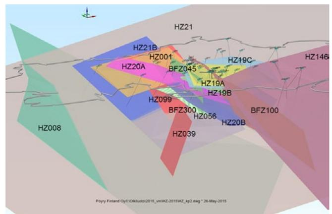
**Figure 3.** Visualisation of the hydrogeological structure model of Olkiluoto. Coloured polygons represent hydrogeological zones (HZ+number) or brittle deformation zones (BFZ+number), the thick grey line the shoreline of Olkiluoto, and thin black lines deep drillholes. View from the south-west.
