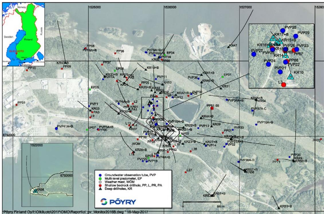
**Figure 1.** Aerial photograph of the Olkiluoto repository site with drillholes and other monitoring points. The surface projections of deep “KR” drillholes are shown as black curves. Grid size 1 km. Insert in the upper left-hand-side corner presents the location of Olkiluoto in Finland.
