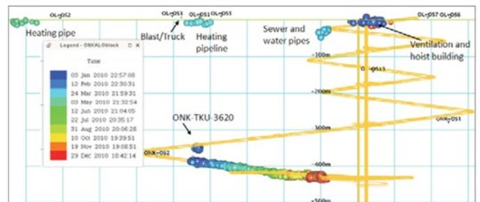
**Figure 2.** Microseismic events detected near the ONKALO in 2010 [13]. Grid size is 100 m × 100 m and the colour scale indicates time of the event from January (blue) to December (red). The ONKALO access ramp and shafts are shown in orange.
