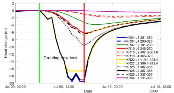
**Figure 6.** Change of hydraulic head in some monitored drillhole sections during a leak from a shaft grouting hole intersecting the HZ20 structure. The vertical green and red lines mark the beginning and end of the leak, respectively. Drillhole section labels consist of drillhole code (KR+number), section code (L+number), and range of drillhole length in metres.
