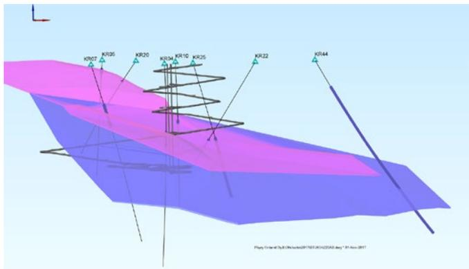
**Figure 4.** 3D illustration of the ONKALO (grey), hydrogeological zones HZ20A (purple) and HZ20B (blue), and some head monitoring sections of drillholes where responses to the leaks discussed in the text were detected. The drillholes are presented with black lines and the selected monitoring sections with thick blue lines. The spiralling access tunnel is about 5 km long and reaches the depth of 450 m from ground surface. View from the south.
