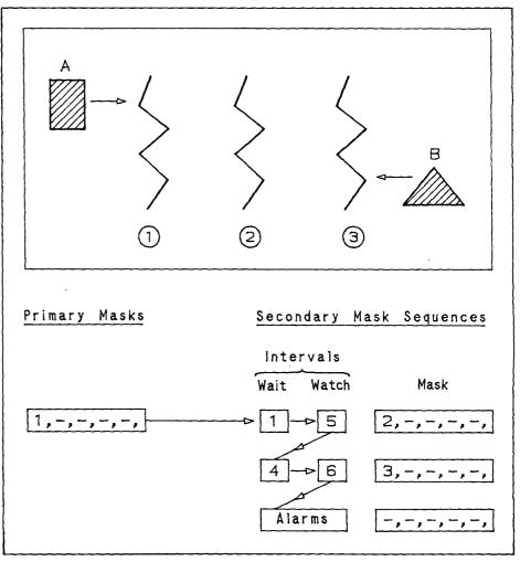
FIG. 5. Simple secondary mask sequence for the detection of objects from left to right
