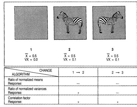
FIG. 4. Examples of scene change detection
