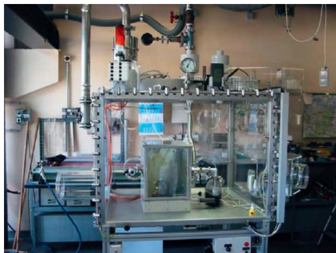
Figure 7: Glove-box for handling of special nuclear material [7].
