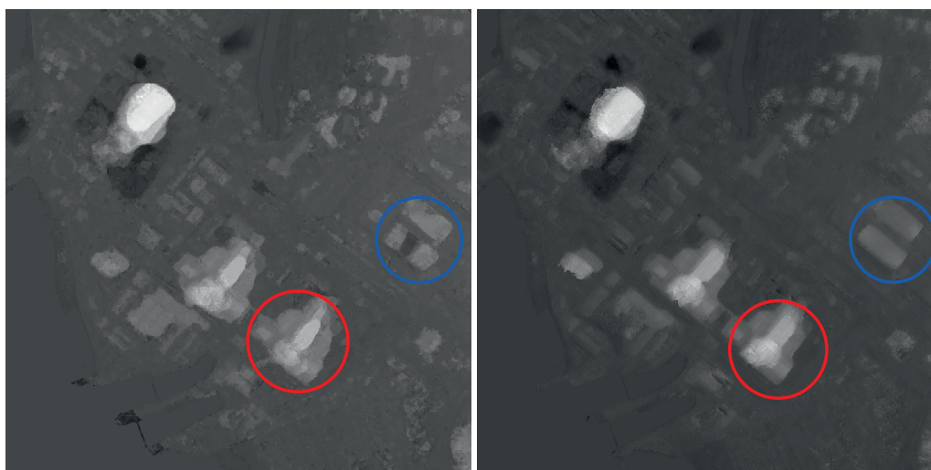
Figure 3: Digital Surface Maps (DSM) of the Olkiluoto site generated with the Joanneum RSG/Impact software from an Ikonos stereo pair (2008).
