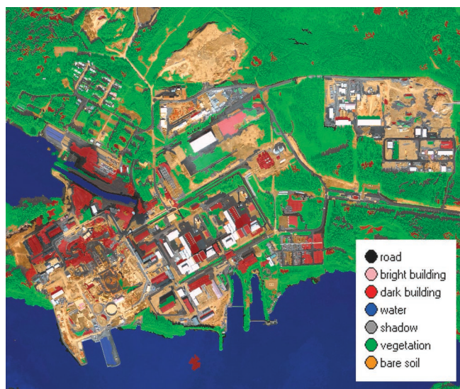
Figure 11: Results of the object-based classification of the Quickbird scene acquired over Olkiluoto in September 2007.
