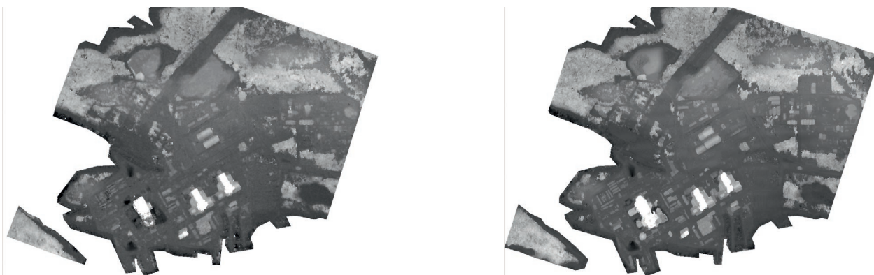
Digital Surface Map (DSM) of the Olkiluoto site from an Ikonos stereo pair acquired in 2008 (left) and a GeoEye-1 stereo pair acquired in 2009 (right)
