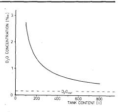
Figure 4 Dependence of the  $D_2O$  concentration on the tank content after addition of 0.25 litre  $D_2O$  with a content of 99.75%
