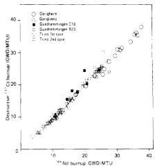
Figure 6 Correlation between <sup>137</sup>Cs and <sup>148</sup>Nd burnups for all JRC samples
