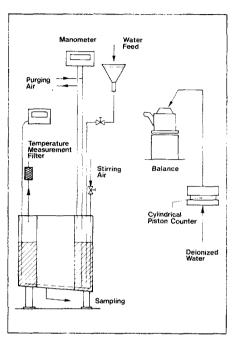
Figure 1 Set-up for calibration of a head-end tank, type WAK
