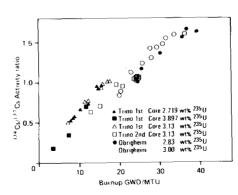
**Figure 5** Correlation between the activity ratio <sup>134</sup>Cs/<sup>137</sup>Cs and burnup for the PWR samples analysed at the JRC
