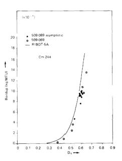
Figure 4 Comparison between calculated and experimental results for Trino Vercellese
