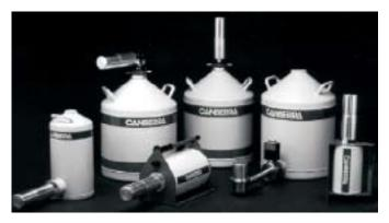
Germanium detectors with dewars for liquid nitrogen cooling
