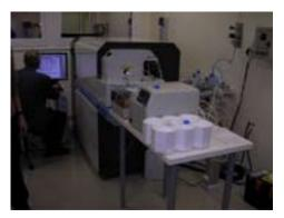
Fig. 3: ICP-SFMS Element2 with ARIDUS sample introduction unit
