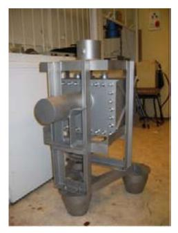
Fig. 1: Underwater Verifier to be used for assay of damaged spent fuel at Paks NPP
