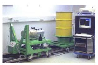
Figure 1 : gamma spectrometry system
