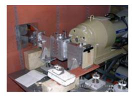
Fig. 5: Cold neutron beam exit used for PGAA
