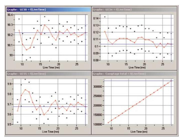
Picture 2: example of a plot during the acquisition of a uranium sample. (Y-axis unit for each isotope: Mass %)
