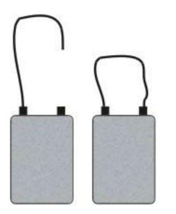
Sealing principle: fibre optic cable/wire "open" or "closed"
