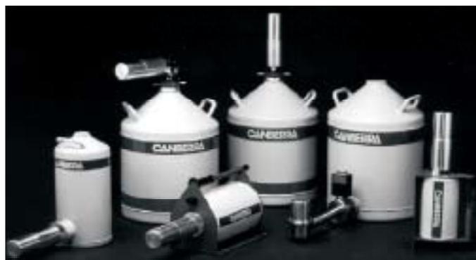
Germanium detectors with dewars for liquid nitrogen cooling
