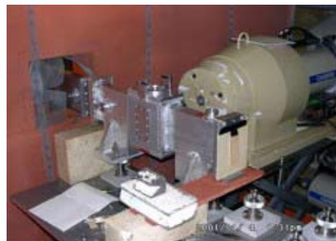
Fig. 5: Cold neutron beam exit used for PGAA
