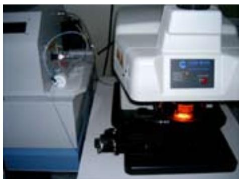
Fig. 4: ICP-SFMS Element2 with Laser Ablation unit
