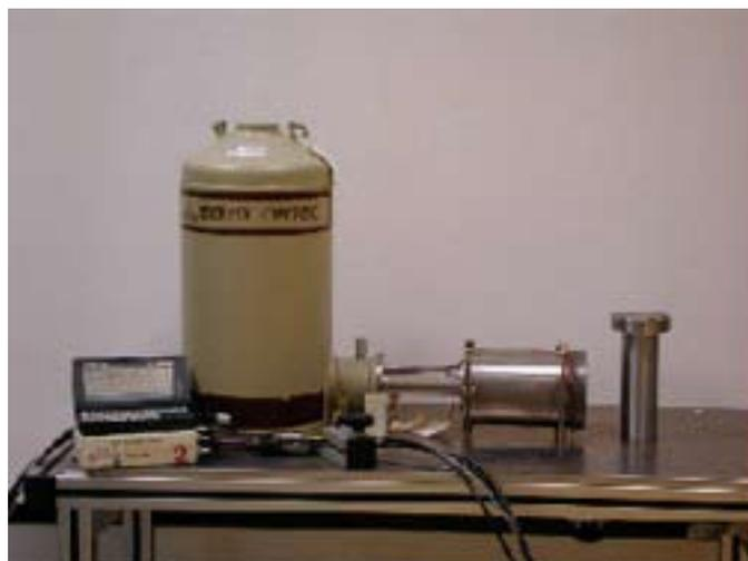
Gamma spectrometer with liquid nitrogen-cooled germanium detector, Mini Multi-channel Analyser, and Hewlett Packard LX200 palmtop computer
