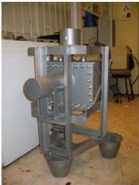
**Fig. 1: Underwater Verifier to be used for assay of damaged spent fuel at Paks NPP**
