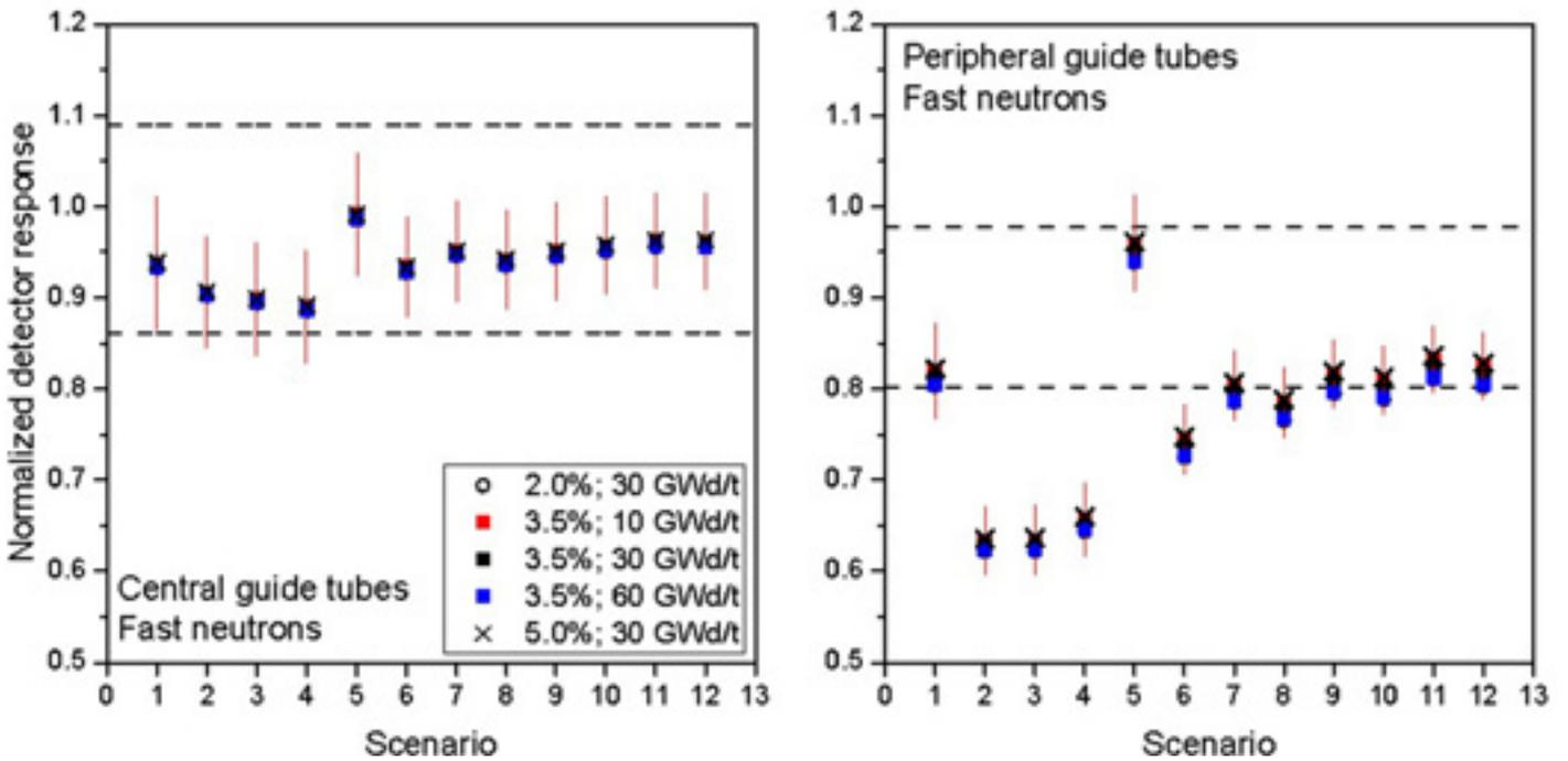
**Figure 6:** Normalized detector responses for fast neutrons in the different diversion scenarios. The average value for central guide tubes (left), and peripheral guide tubes (right) are shown. The lower and upper boundaries for the cases with complete fuel assemblies are also reported.
