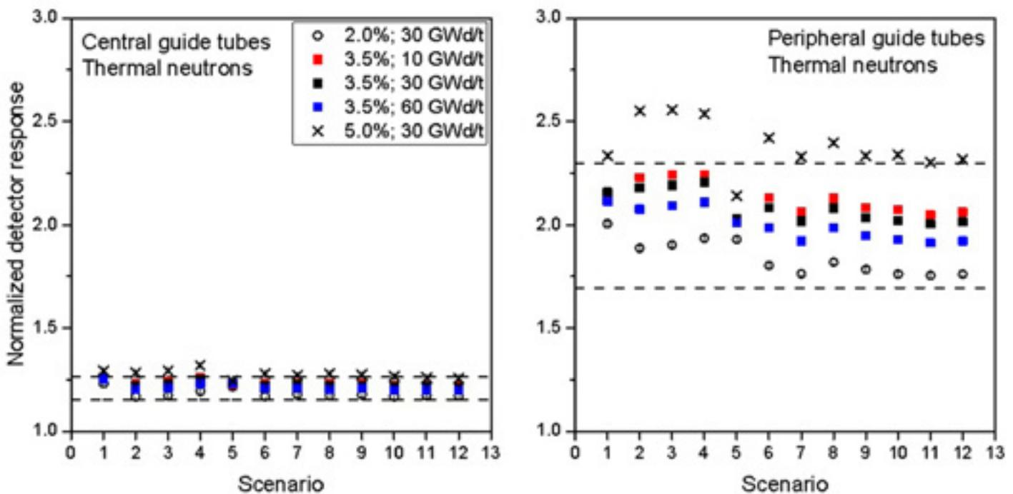
**Figure 4:** Normalized detector responses for thermal neutrons in the different diversion scenarios. The average value for central guide tubes (left), and peripheral guide tubes (right) are shown. The lower and upper boundaries for the cases with complete fuel assemblies are also reported.
