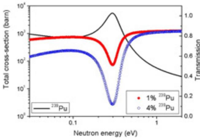
**Figure 1:** Total cross-section of  $^{239}\text{Pu}$  and transmission of a neutron flux through samples containing  $^{239}\text{Pu}$ . The cross-section values were obtained from the ENDF/B-VII.0 data library, whereas the transmission was calculated with Monte Carlo simulations.
