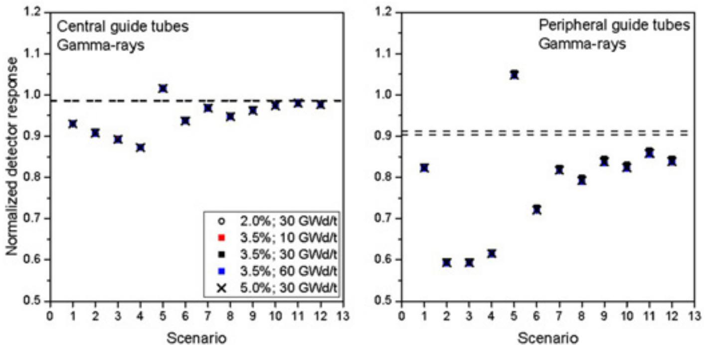
**Figure 7:** Normalized detector responses for gamma-rays in the different diversion scenarios. The average value for central guide tubes (left), and peripheral guide tubes (right) are shown. The lower and upper boundaries for the cases with complete fuel assemblies are also reported.
