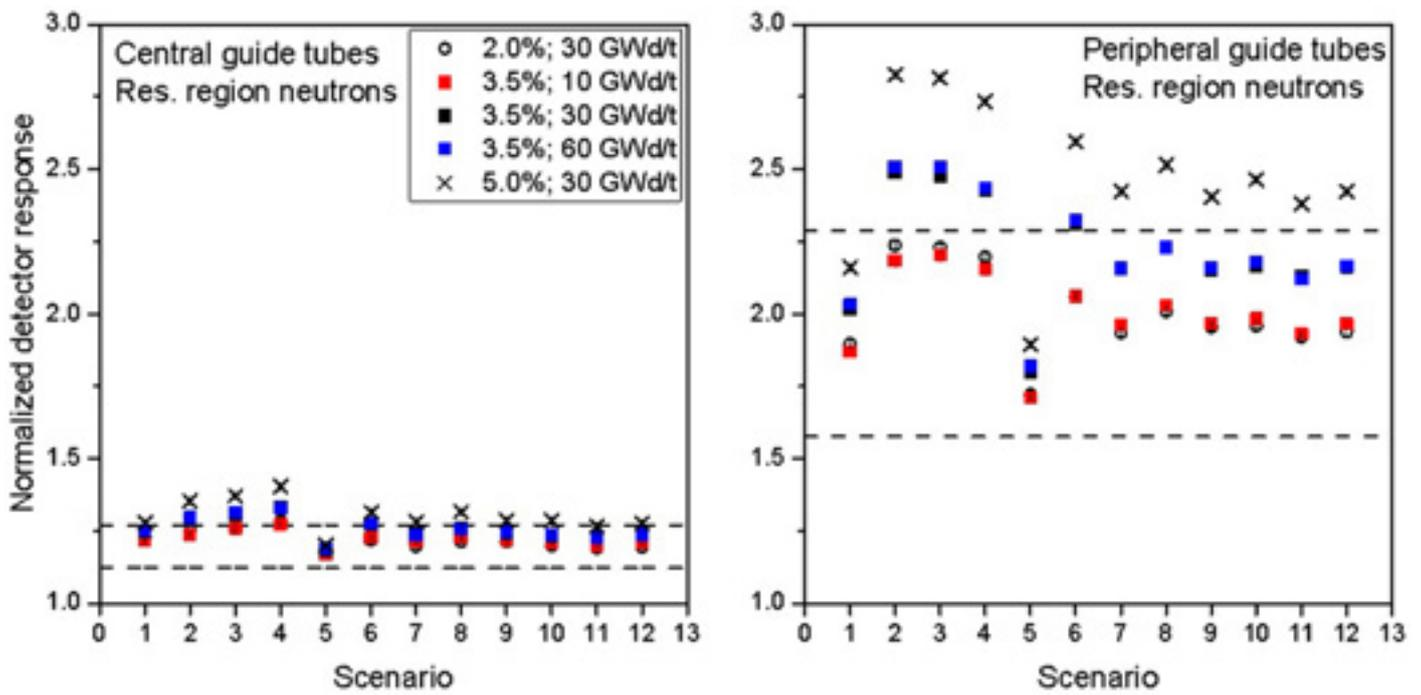
**Figure 5:** Normalized detector responses for neutrons around the 0.3 eV resonance region in the different diversion scenarios. The average value for central guide tubes (left), and peripheral guide tubes (right) are shown. The lower and upper boundaries for the cases with complete fuel assemblies are also reported.
