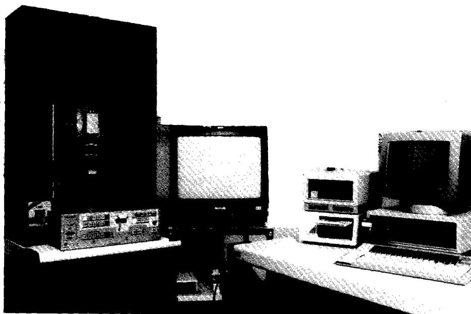
FIG. 7. Computer vision system for seal verification
