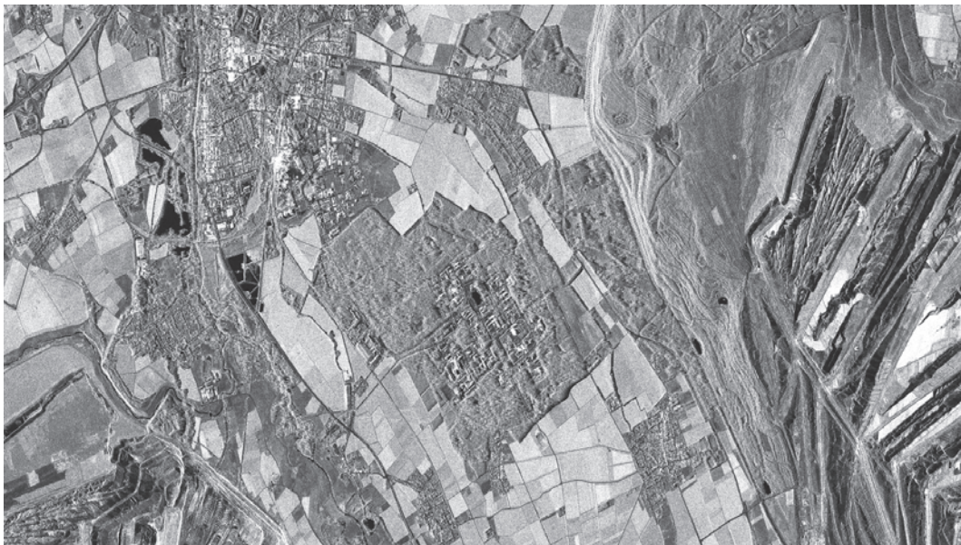
Figure 1: Example of the amplitude information of a single High-Resolution Spotlight TerraSAR-X scene, presented in range (horizontal) and azimuth (vertical) coordinates.
