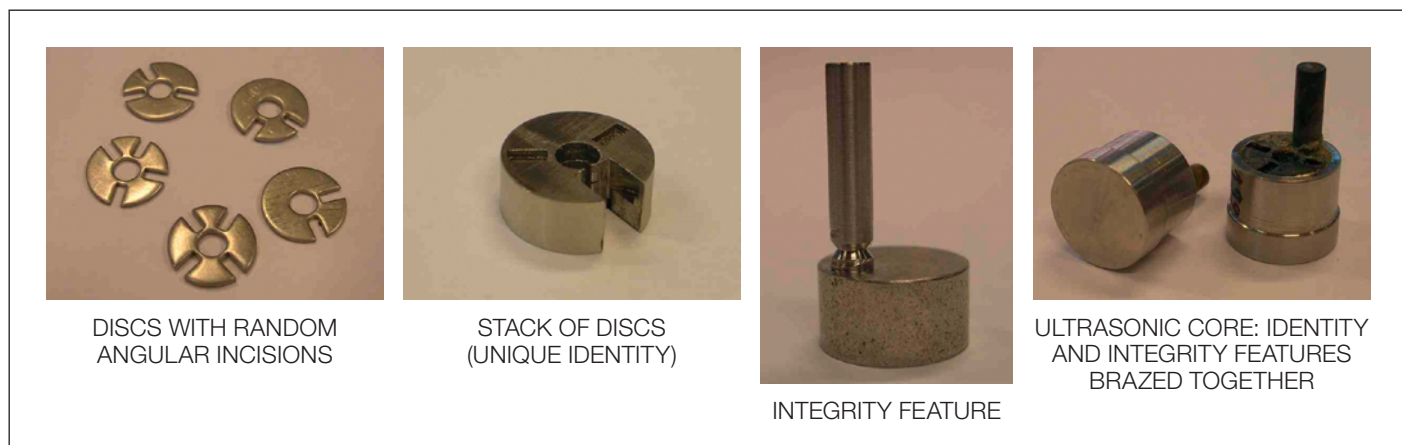
Figure 8: Core of ultrasonic seals.
