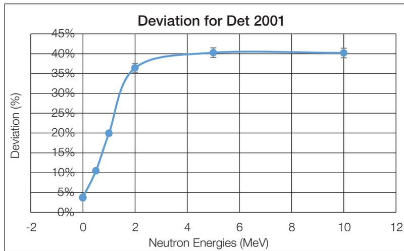
**Figure 8:** Deviation for detector 2001 in terms of neutron energy. Note how the deviation increases rapidly as neutron energy increases. Here deviation shows the degree of deviation from the case of non-diversion.
