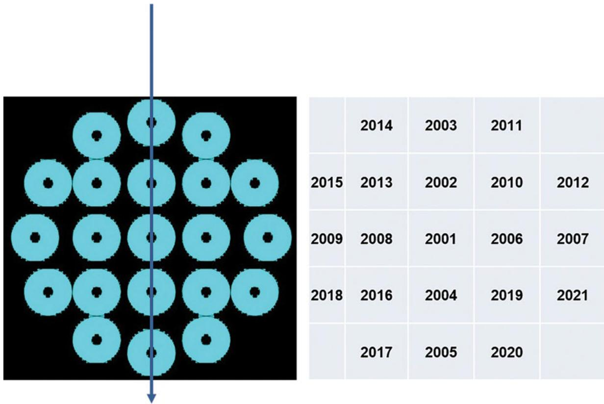
**Figure 5:** The left figure indicate how data were read and shown as a graph later for easy analysis and results presentation. The numbers in the right figure indicate neutron tally (detector) number which is essentially relative neutron flux.
