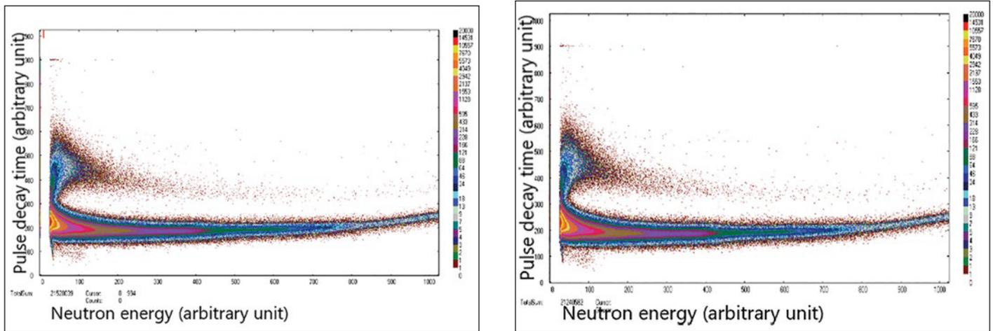
**Figure 10:** PSD plots obtained with the stilbene scintillator using PSD electronics for the case of Cf source placed directly below the detector and the source off the collimator position. The radiations were attenuated by 38 cm of steel. The upper neutron band signals were well separated from the lower gamma band signals.
