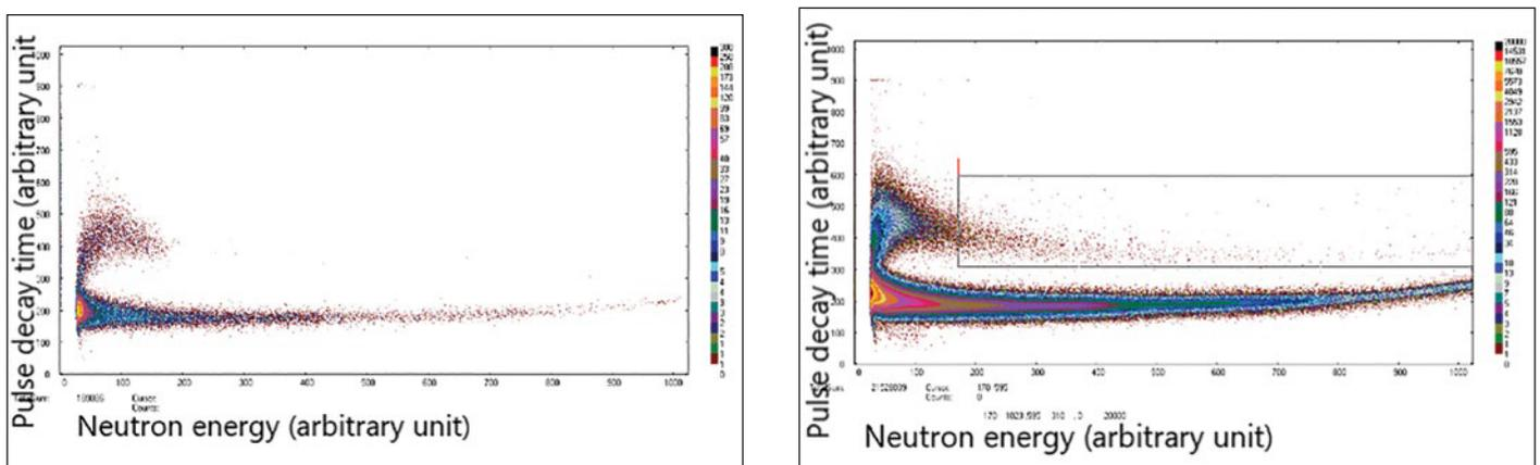
**Figure 11:** PSD plot in the left obtained with the stilbene scintillator using PSD electronics and DD 2.4 MeV neutrons. Note that there is a distinctive end of neutron band, showing a feature that can be useful to separate neutron signals. The information is used to select a rectangular ROI that predominantly has neutrons with energy greater than approximately 2.4 MeV. An example of ROI selection is shown in the right plot.
