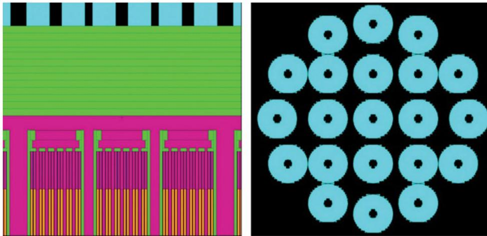
**Figure 4:** Close up cross-sectional view of MCNP set up. The neutron detectors with poly around them are positioned on the top surface of the CASTOR 21. Every detector is located directly above the center of the PWR spent fuel assembly.
