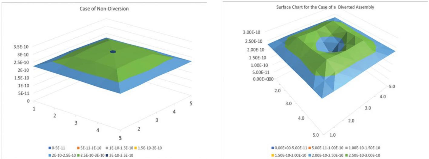
**Figure 6:** The left figure is obtained for the case of non-diversion. The right figure is for the case where the center assembly was replaced with a dummy stainless steel assembly. Note the deviation in the center in the right figure.
