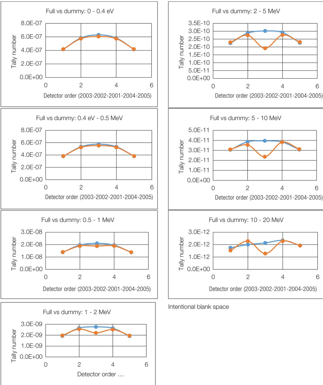
**Figure 7:** Vertical tally profiles, i.e., detector tally through 2003-2002-2001-2004-2005, as the energy tally bin increases.- The blue curve is the cask with all 21 assemblies and the orange curve is when the center assembly has been replaced with a stainless steel dummy assembly.
