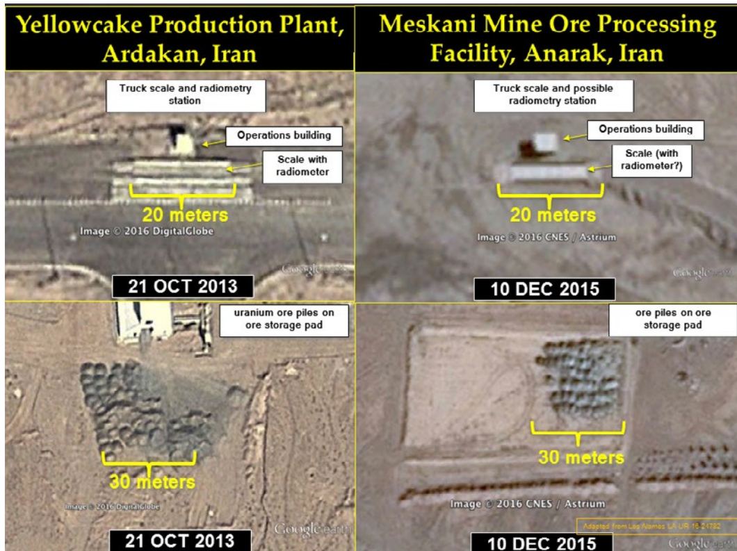
Figure 6: Late-2015 overview of the new small ore processing facility serving the newly re-activated, adjacent, Meskani mine. Labels identify the more likely roles of each part of the facility for illustrative purposes and are not meant to be definitive.
