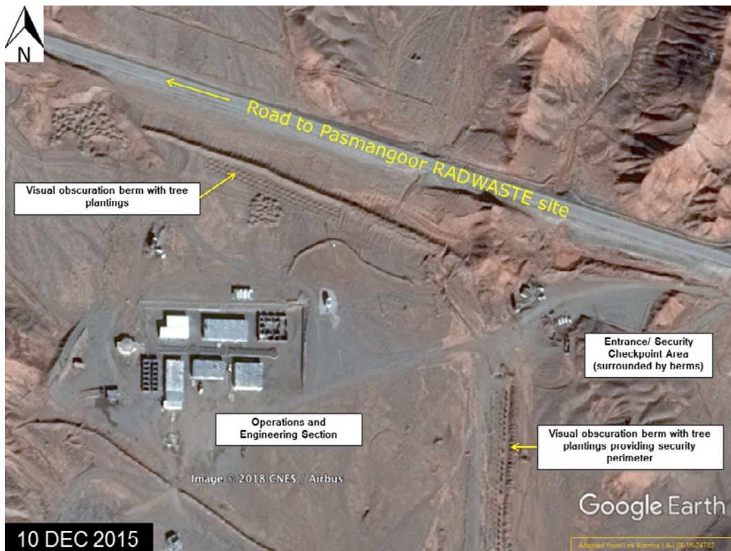
Figure 10: Operations and Engineering Section of the new ore processing facility showing the physical security as exemplified by an entrance/checkpoint area and visual obscuration berms that also serve as perimeter security barriers. Tree plantings (three rows of dot-like features) inside the berms are also evident, which will help with berm stabilization as well as providing additional future visual obscuration.
